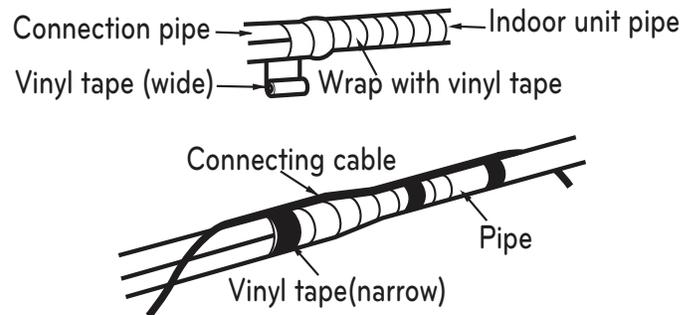
Figure 67: Cutaway of Proper Bundling.
