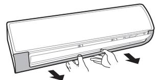
Figure 18: Releasing the Sides of the Bottom Panel.
