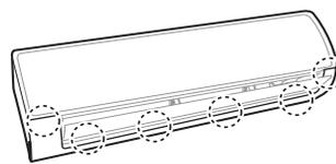
Figure 17: Releasing the Back of the Bottom Panel.
