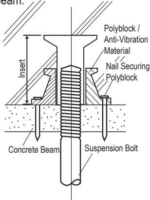
Figure 7: Close up of Bolt Attachment.
