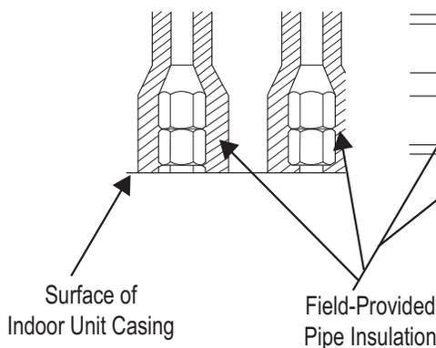
Figure 70: Typical Refrigerant Flare Fitting Insulation Detail.
