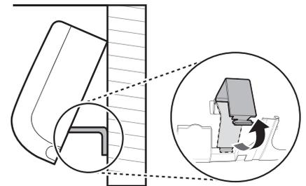
Figure 46: Connecting the Refrigerant Field Piping to the Indoor Unit Piping.
