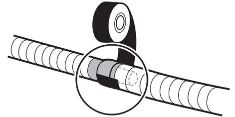
Figure 60: Insulating the Indoor Unit to Extension Drain Hose Connection.
