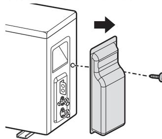
Figure 99: Accessing the LAU150HYV3 / LAU180HYV3 / LAU240HYV3 Outdoor Unit Terminal Block.
