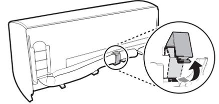
Figure 45: Using the Piping Holder to Prop the Indoor Unit Away from the Wall.
