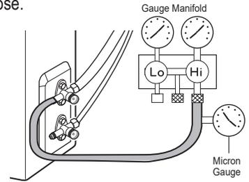
Figure 126: Closing the Outdoor Unit Liquid Piping Service Valve.
