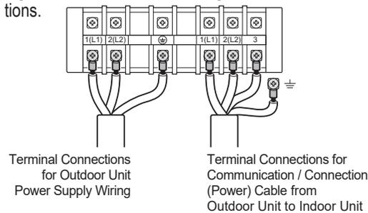
Figure 103: LAU090-120HYV3 Outdoor Unit Conduit Assembly.
