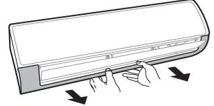
Figure 39: Releasing the Sides of the Bottom Panel.
