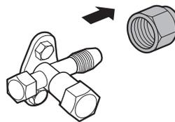
Figure 36: Connecting the Flared Field Piping to the Outdoor Unit Connection.
