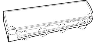
Figure 38: Releasing the Back of the Bottom Panel.
