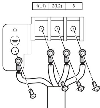
Figure 92: Securing the Cable Clamp.
