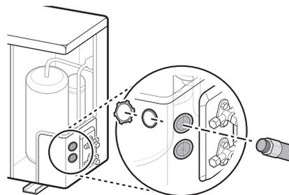
Figure 102: Outdoor Unit Wiring / Cable Connections.
