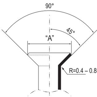
Flared Connection Dimensions / Tightening Torque.
