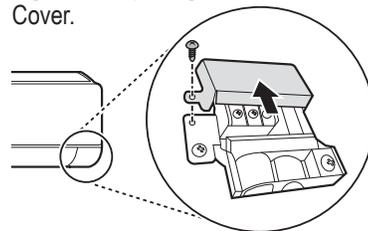
Figure 90: Opening the Cable Clamp.
