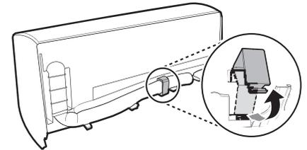
Figure 41: Properly Unfolding and Bending the Piping.
