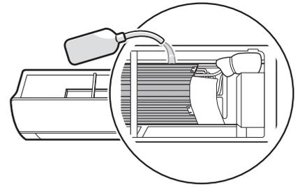
Figure 65: Checking for Leaks at the Connection Areas.
