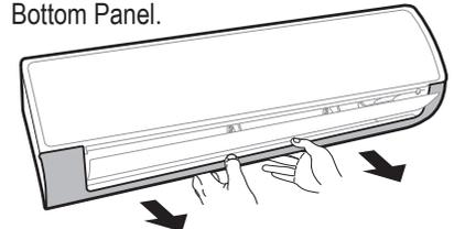
Figure 87: Releasing the Sides of the Bottom Panel.
