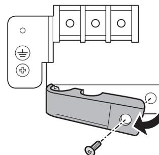
Figure 93: Closing the Control Box Cover.
