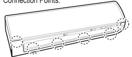
Figure 86: Releasing the Back of the Bottom Panel.
