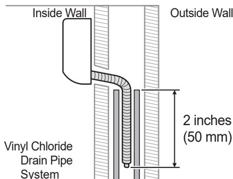
Figure 62: Inserting the Drain Hose More Than Two (2) inches Into the Wall-Embedded Drain Pipe System (Close Up View).
