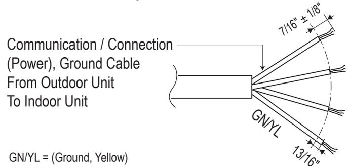
Figure 81: Typical Single Zone Power / Communication System Diagram.
