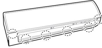
Figure 118: Reconnecting the Back of the Bottom Panel.
