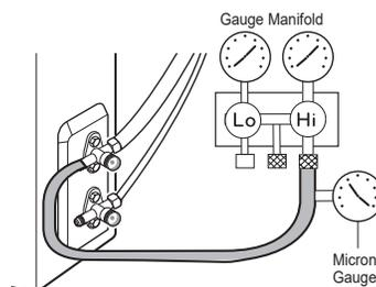
Figure 112: Opening the Outdoor Unit Service Valves Counter-clockwise.
