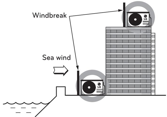
Figure 3: Placement Using Building as Shield.
