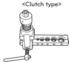
Firmly hold copper tube in a bar(or die) as indicated dimension in the table above.
