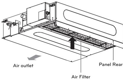
Low static duct type in case of suction from bottom side.
