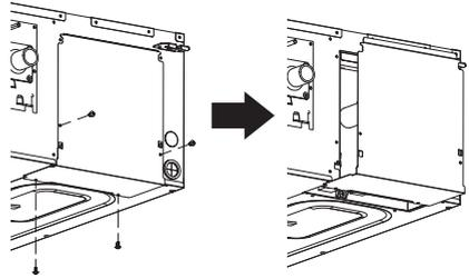
After remove the control box cover, insert cables onto the bush and conduit and then connect at terminal block.
