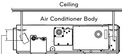
Keep the length of the bolt from the bracket to 50 mm (1-31/32 Inch) or less
