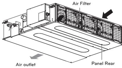
Low static duct type in case of suction from back side.
