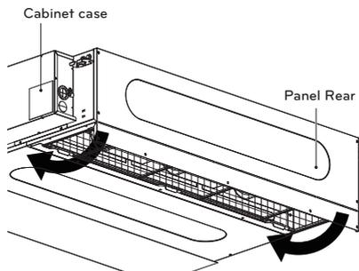
In case of suction from bottom size, bend the Panel rear and screw with cabinet case.
