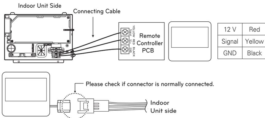
Please use extension cable if the distance between wired remote controller and indoor unit is more than 10 m (32-4/5 ft).
