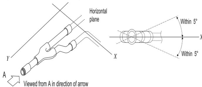
Figure 58: Y-Branch Port Identifier Diagram.
