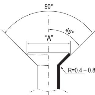
Flared Connection Dimensions / Tightening Torque.
