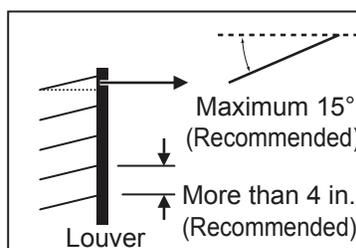
Figure 9: Using “S” Type Louvers.
