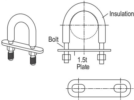
Figure 36: O-Ring Support with Insulation.
