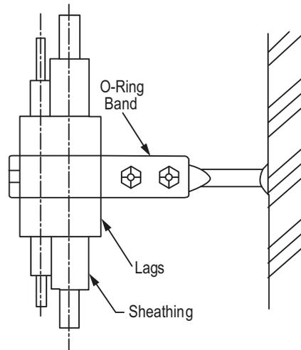
Figure 40: One-Point Down-Stop Support (>441 lbs.).
