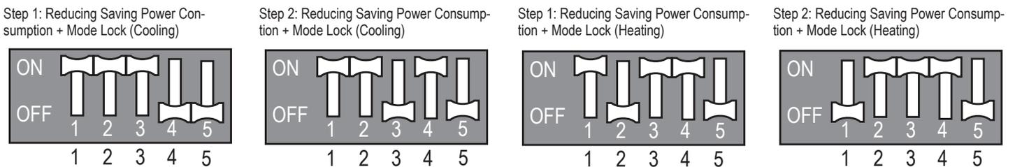
Figure 123: LMU483-543-601HV Saving Power Consumption with Mode Lock DIP Switch Settings.
