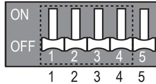
Figure 112: LMU483-543-601HV Outdoor Unit DIP Switches (in Normal Operation Setting).
