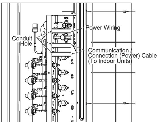
Figure 72: Location of the Power Wiring and Communication Cable Terminals LMU483-543-601HV).
