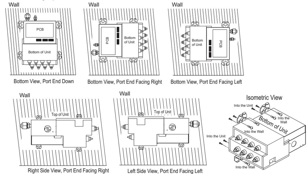
Figure 23: Unacceptable Branch Distribution Unit Wall Mount Orientations.
