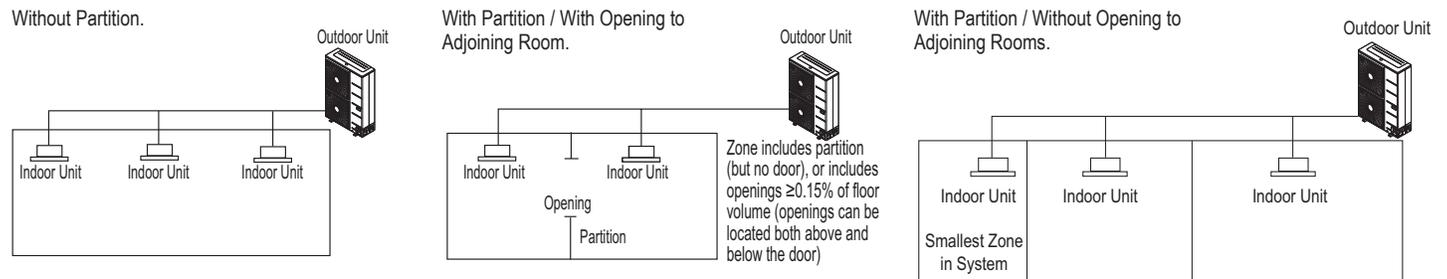
Figure 107: Example of Acceptable Ventilation Methods.
