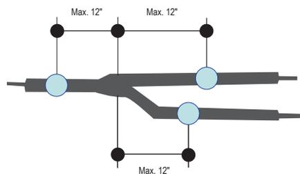
Figure 34: Pipe Support at Header Fitting.
