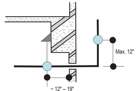
Figure 32: Pipe Support at Indoor Unit.
