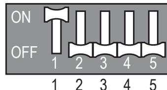
Figure 115: LMU483-543-601HV Forced Cooling DIP Switch Setting.
