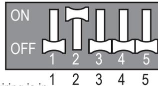
Figure 117: LMU483-543-601HV Wiring Error Check DIP Switch Setting.
