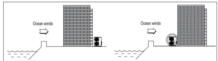
If the outdoor unit must be placed in a location where it would be subjected to direct ocean winds, install a concrete windbreaker strong enough to block any winds. Windbreaker height and width must be more than 150% of the outdoor unit, and be installed at least 27-1/2 inches away from the outdoor unit to allow for airflow.
