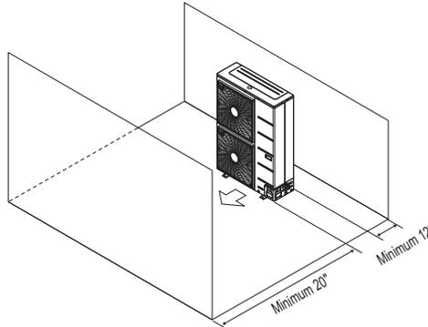
Where there are obstacles on both suction and discharge sides (discharge side obstacle is lower than the outdoor unit).
