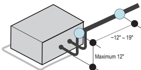
Figure 33: Pipe Support at Y-branch Fitting.
