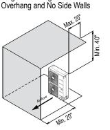
Side by Side—High Front Wall with No Side Walls Side by Side—High Front Wall with Building Overhang and No Side or Rear Walls
