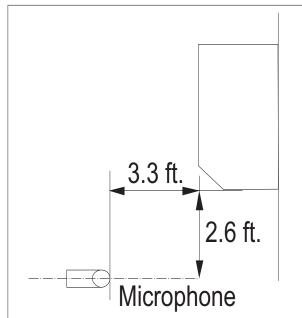
Measurement taken 2.6' below the bottom of the unit and at a distance of 3.3' from face of unit.
