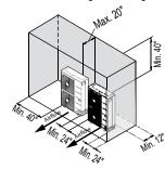
Figure 256: Proper Outdoor Unit Placement and Clearances When There Are Obstacles on the Discharge Side. Single Unit—High Front Wall with Building
