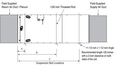
Table 110: Bracket / Bolt Position Dimensions for Horizontal Left and Horizontal Right Installation.
