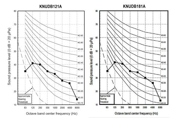
Figure 188: KNUDB121A and KNUDB181A Sound Pressure Level Diagrams.
