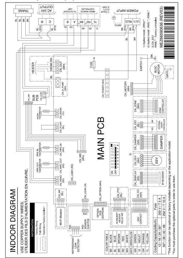
Figure 225: Multi Position Air-Handling Indoor Unit Wiring Diagram for KNMLB121A, KNMLB181A, KNMLB241A.
