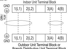
Branch Distribution Unit Terminal Block (Multi F MAX Systems Only) Figure 243: Connecting the Power Wiring and Communications Cable.
