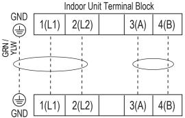
Outdoor Unit Terminal Block or Branch Distribution Unit Terminal Block (Multi F MAX Systems Only)
