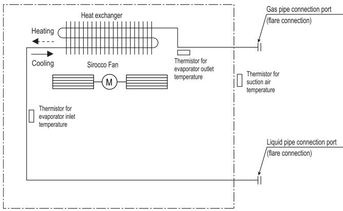
Figure 159: KNUJB301A and KNUJB361A Refrigerant Flow Diagram.
