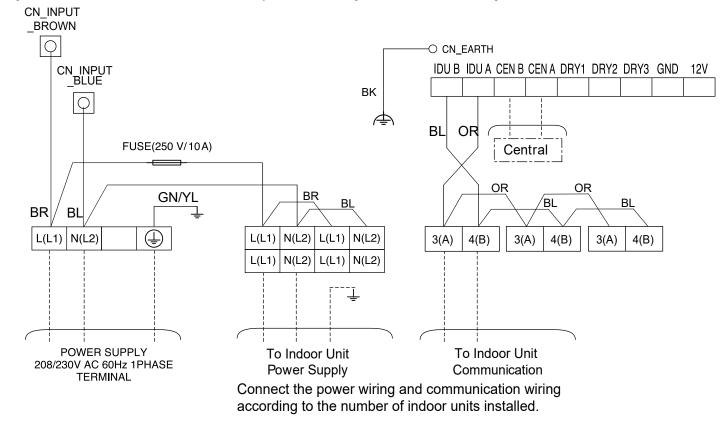
Figure 268: Multi F KUMXB301A and KUMXB361A System Power Wiring and Communications Wiring.
