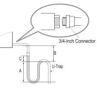
Figure 238: Installing the U-Trap.
