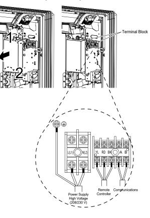
Figure 81: Securing Wiring to Unit.
