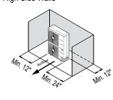
Single Unit—High Rear Wall with Building Overhang
