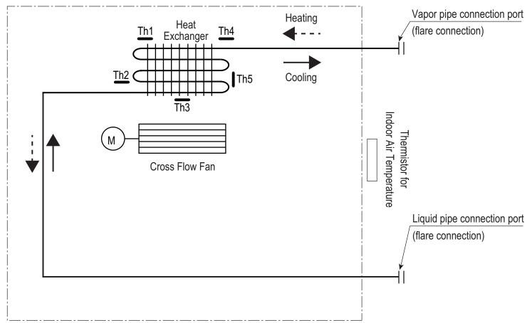
Figure 40: Multi F High Efficiency Wall-Mounted Indoor Unit Refrigerant Flow Diagram.
