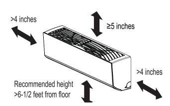
Figure 10: Minimum Clearance Requirements.
