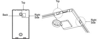
Figure 27: Attaching the Wall Plate.
