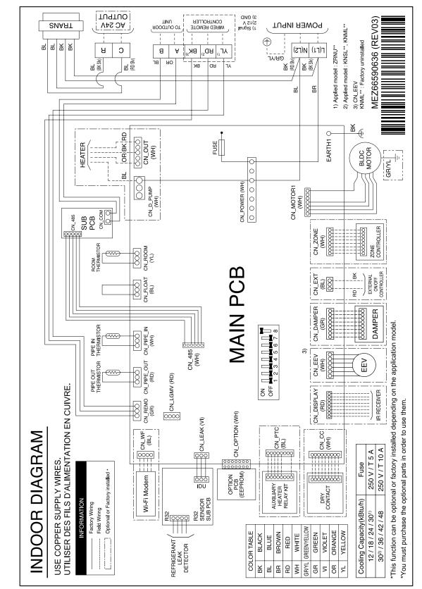
Figure 226: Multi Position Air-Handling Indoor Unit Wiring Diagram for KNMLB301A, KNMLB361A.
