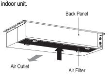
Figure 99: Air inlet from the bottom of the
