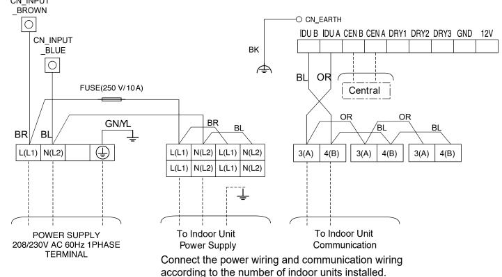
Figure 270: Multi F with LGRED KUMXA181A, KUMXA241A, and KUMXA301A System Power Wiring and Communications Cable.
