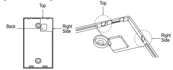
Figure 149: Attaching the Wall Plate.
