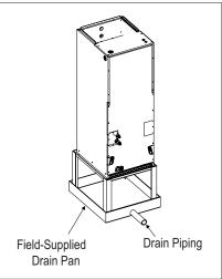
Figure 236: Typical Horizontal Left/Right Installation Drain System.
