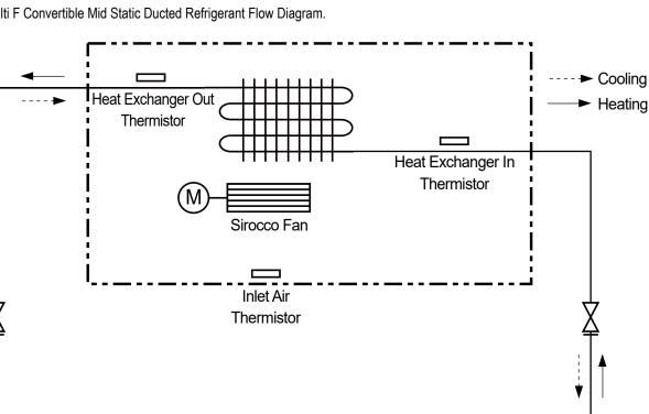
Figure 126: Multi F Convertible Mid Static Ducted Refrigerant Flow Diagram.
