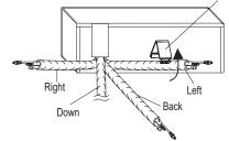
Figure 52: Piping Installed to the Right.
