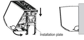
Figure 14: Locking the Indoor Unit onto the Installation Plate.
