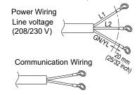
Figure 262: Power Wiring and Communication Wiring from ODU to IDU / BDU (Multi F MAX Only), and from the BDU to the IDU (Multi F MAX Only) GREATER THAN 130 feet
