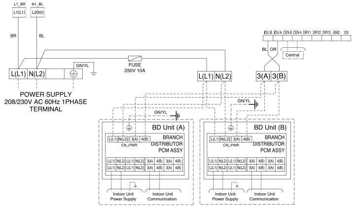
Connect power wiring and communications wiring according to the number of indoor units installed.
