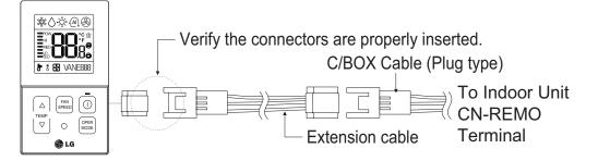
Figure 246: Wired Controller Connection on the Indoor Unit Terminal Block.
