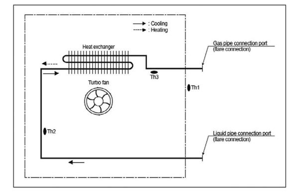
Figure 71: Multi F Low Wall Console Indoor Unit Refrigerant Flow Diagram.
