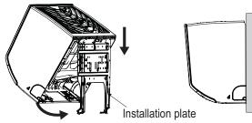
Figure 49: Removing the Frame Cover.
