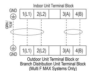
Figure 79: Connecting Power Wiring / Communications Cable.
