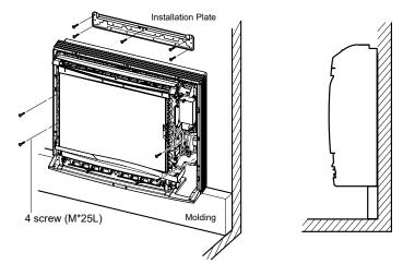
Figure 75: Wall Installation.
