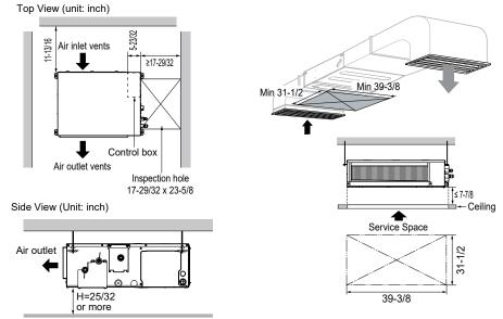
Dimension "H" is necessary for drain slope
