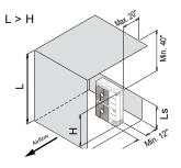
Obstacle Height of Discharge Side Is Lower than the Outdoor Unit.
