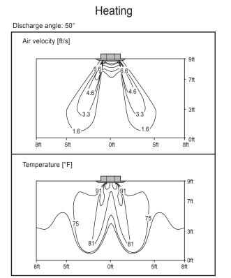
Figure 192: KNUDB181A Air Velocity and Temperature Distribution Charts.
