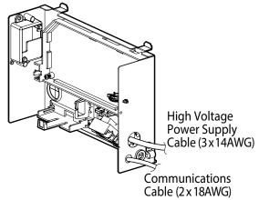
Figure 172: Indoor Unit to Outdoor Unit / Branch Distribution Unit (Multi F MAX systems only) Power Wiring / Communications Cable Connections.
