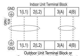
Figure 109: Simplified View of Indoor Unit to Outdoor Unit / Branch
