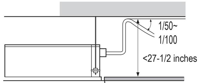
Figure 203: Checking the Drain Pump.
