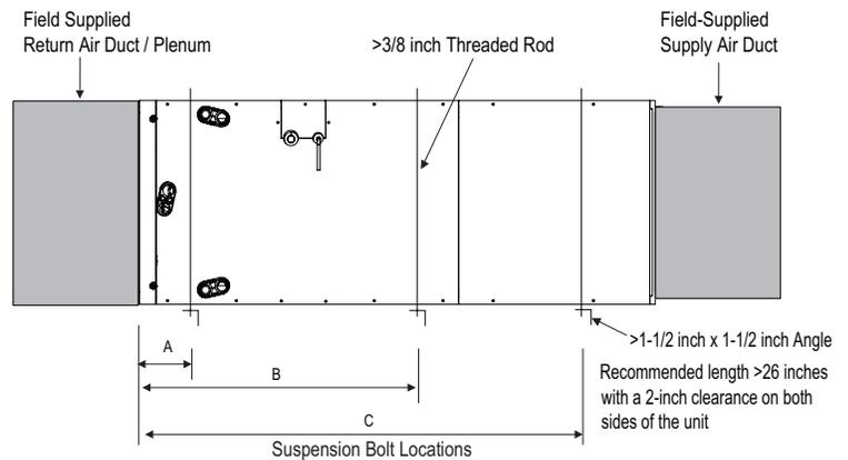
Table 110: Bracket / Bolt Position Dimensions for Horizontal Left and Horizontal Right Installation.
