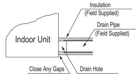
Figure 104: Indoor Unit Using Drain Pump.
