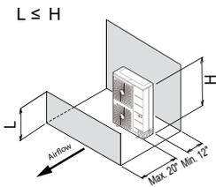
Single Unit—High Rear Wall and Low Front Wall with Building Overhang and No Side Walls
