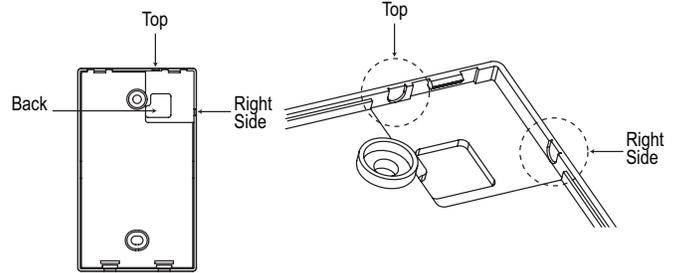
Figure 61: Attaching the Wall Plate.
