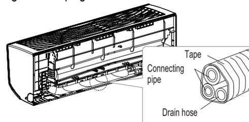
Figure 52: Piping Installed to the Right.
