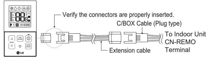
Figure 112: Wired Controller Connections on the Indoor Unit Terminal Block.
