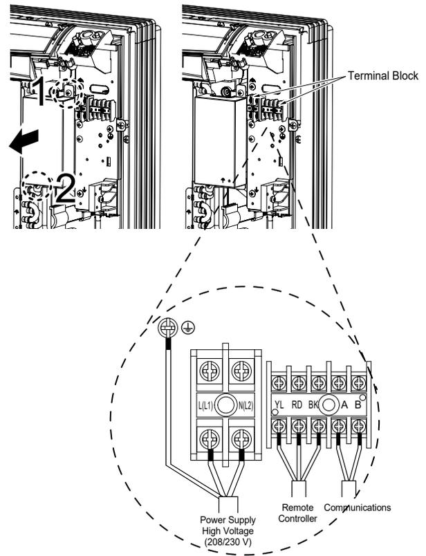
Figure 81: Securing Wiring to Unit.
