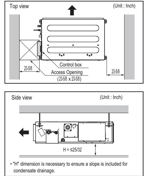
Figure 97: Service / Access Panel Dimensions.
