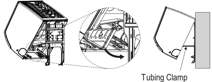
Figure 49: Removing the Frame Cover.
