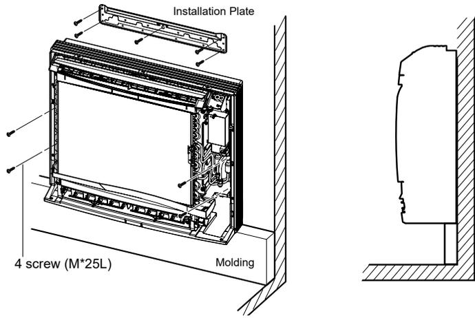
Figure 76: Recessed Installation.
