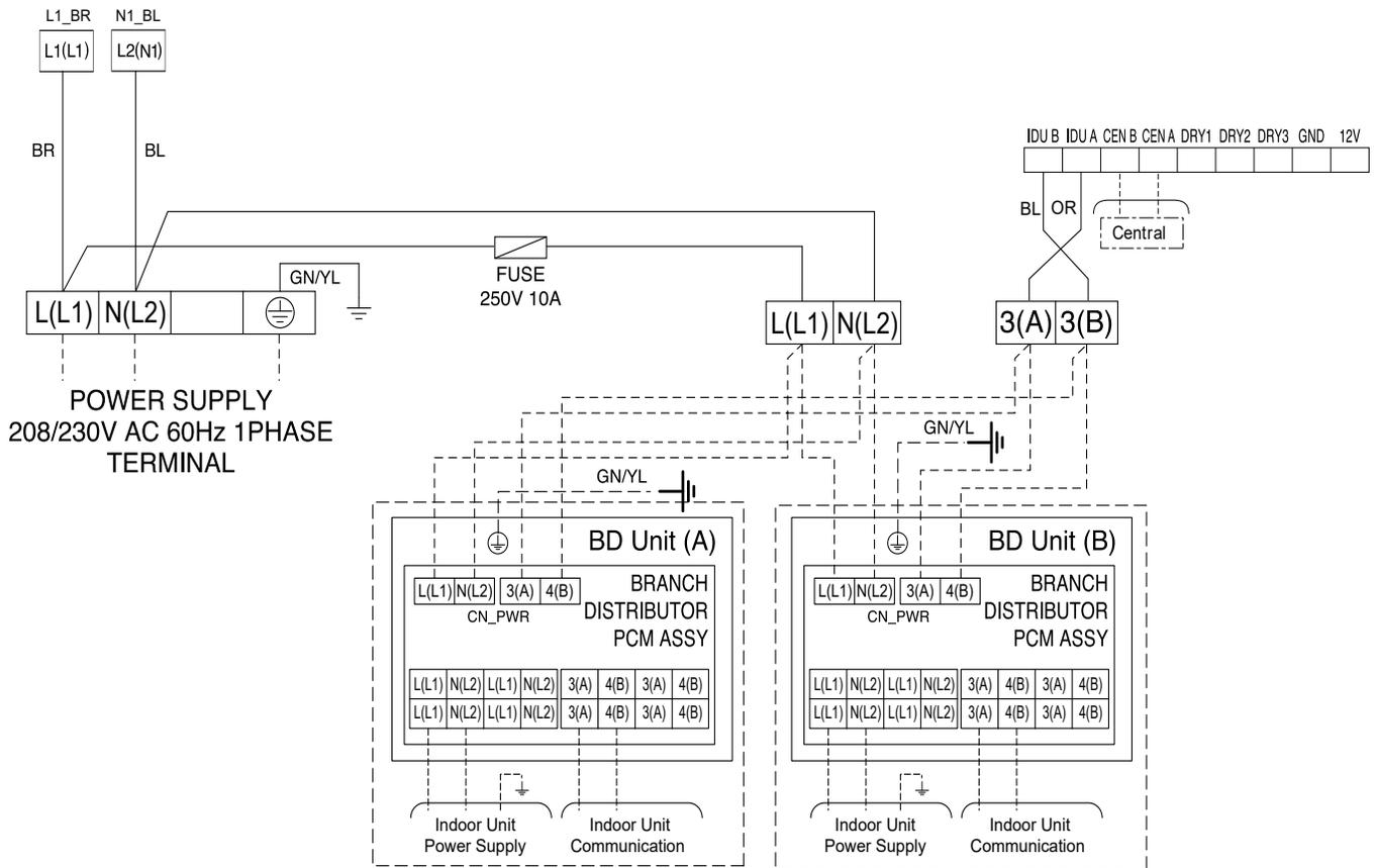
Connect power wiring and communications wiring according to the number of indoor units installed.
