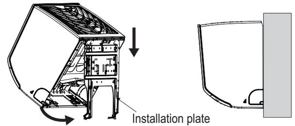
Figure 15: Accessing the Back of the Indoor Unit.
