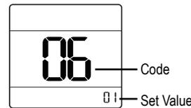
Figure 152: Controller External Static Pressure Setting Display.
