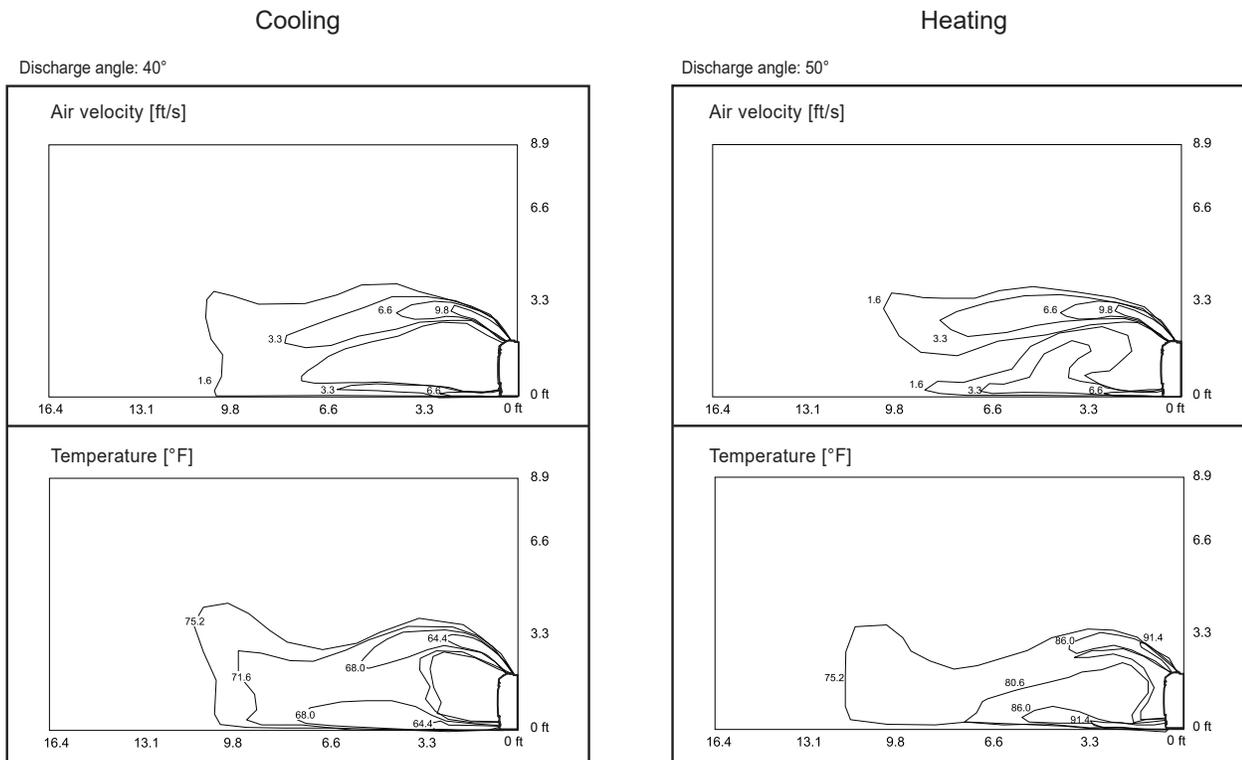
Figure 70: KNMQB151A Air Velocity and Temperature Distribution Charts.
