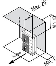
Single Unit—High Rear and Side Walls with Building Overhang
