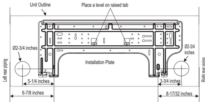
Figure 12: Installation Plate for KNUAK181A Units.
