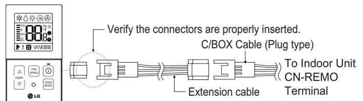
Figure 210: Wired Controller Connections on the Indoor Unit Terminal Block.
