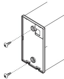
Figure 250: Installing / Removing the Controller.
