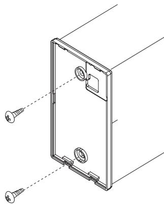
Figure 28: Installing/Removing the Controller.
