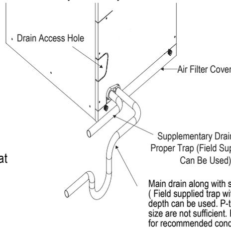
Figure 240: Horizontal Primary and Secondary Drain Layout.
