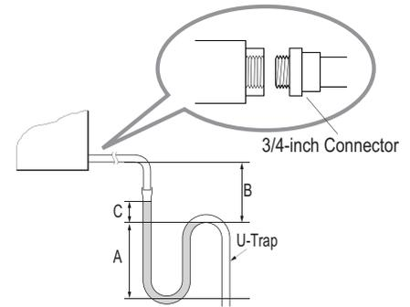
Figure 239: Vertical Primary and Secondary Drain Layout.
