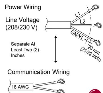
**Multi F / Multi F MAX Power Wiring / Communications Wiring**
