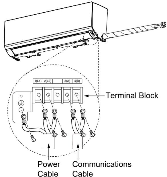
Figure 55: Simplified View of Indoor Unit to Outdoor Unit / Branch Distribution Unit Terminal Connections.
