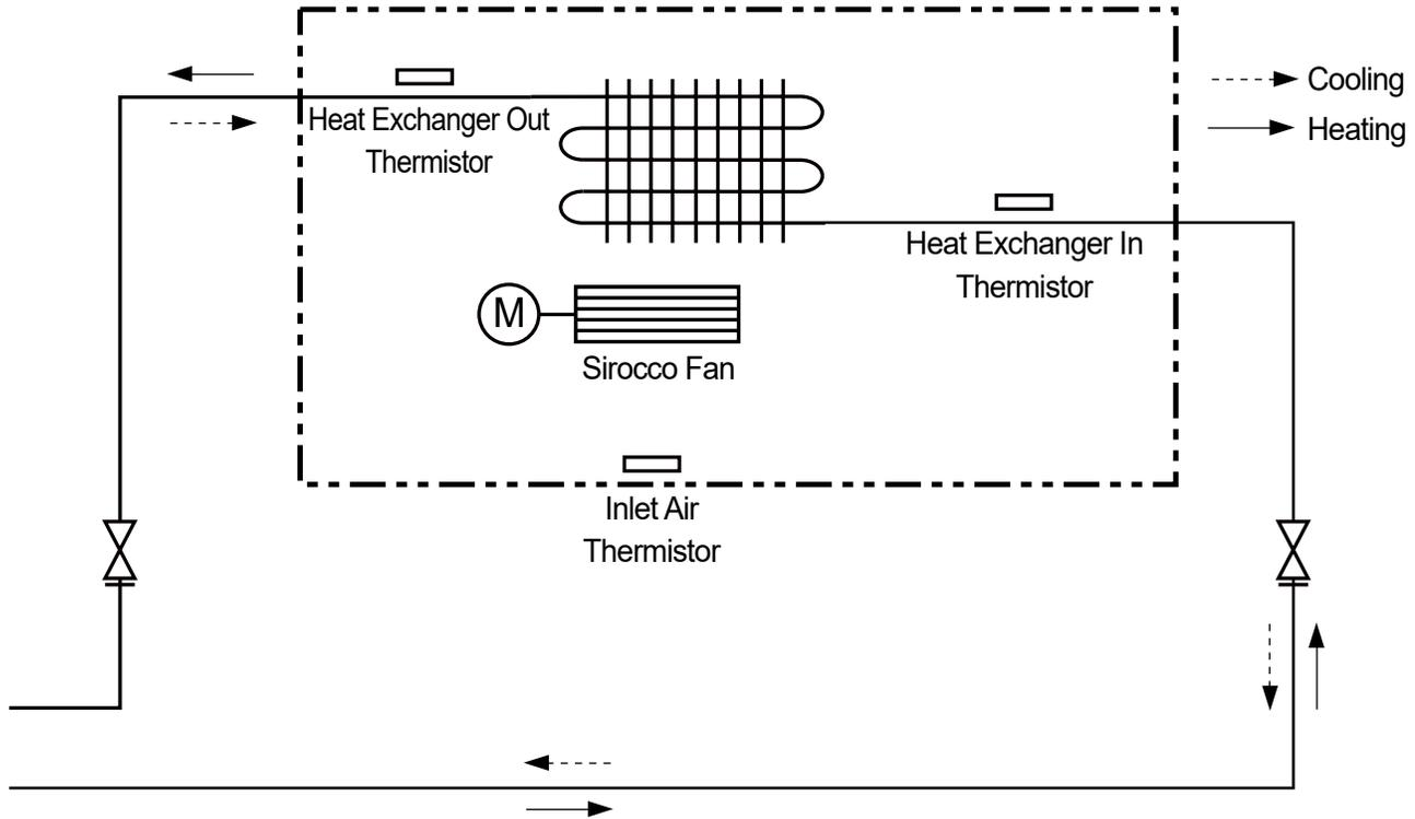
Table 59: Multi F Convertible Mid Static Duct Indoor Units Thermistor Details.
