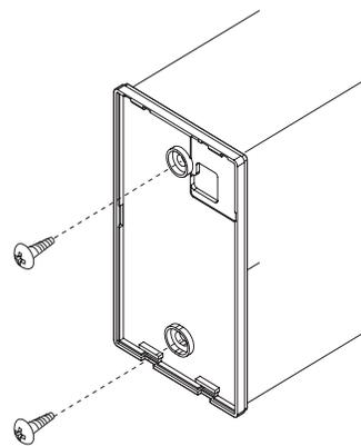
Figure 179: Installing / Removing the Controller.
