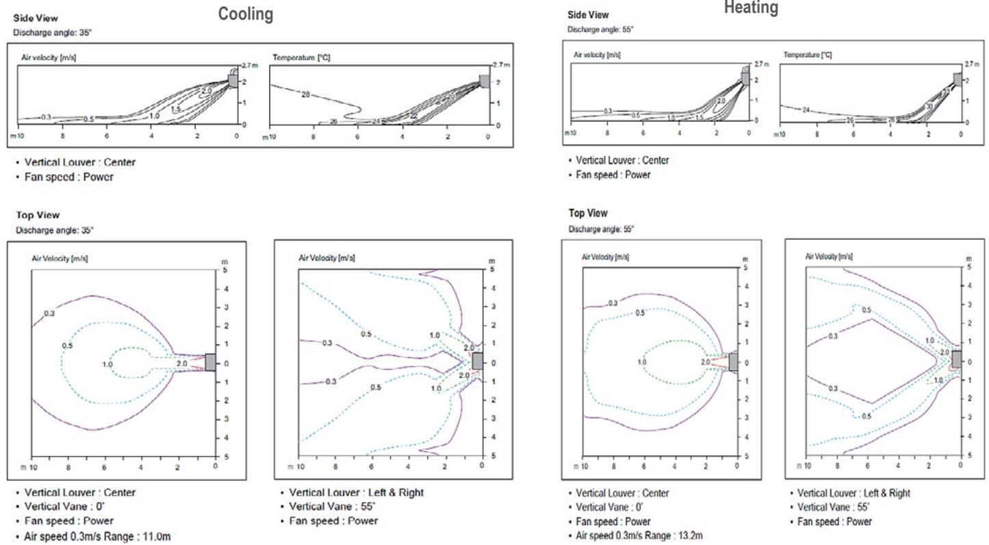
Figure 7: KNUAK181A Air Velocity and Temperature Distribution Charts.
