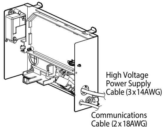
Figure 143: Simplified View of Indoor Unit to Outdoor Unit / Branch Distribution Unit Terminal Connections.
