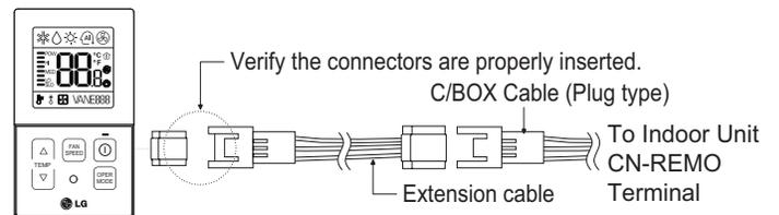
Figure 146: Wired Controller Connections on the Indoor Unit Terminal Block.
