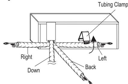
Figure 18: Piping Installed to the Left.
