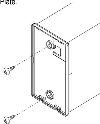
Figure 214: Installing / Removing the Controller.
