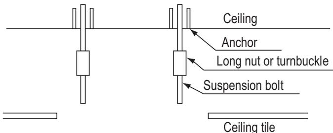
Figure 200: Installation Diagram.
