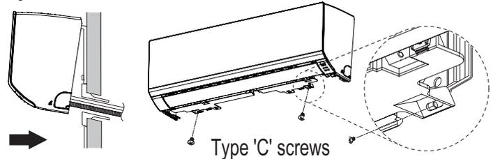
Figure 63: Removing the Filter Tabs.
