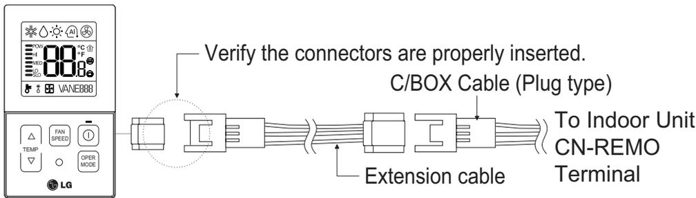
Figure 246: Wired Controller Connection on the Indoor Unit Terminal Block.
