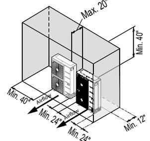
Figure 256: Proper Outdoor Unit Placement and Clearances When There Are Obstacles on the Discharge Side.
