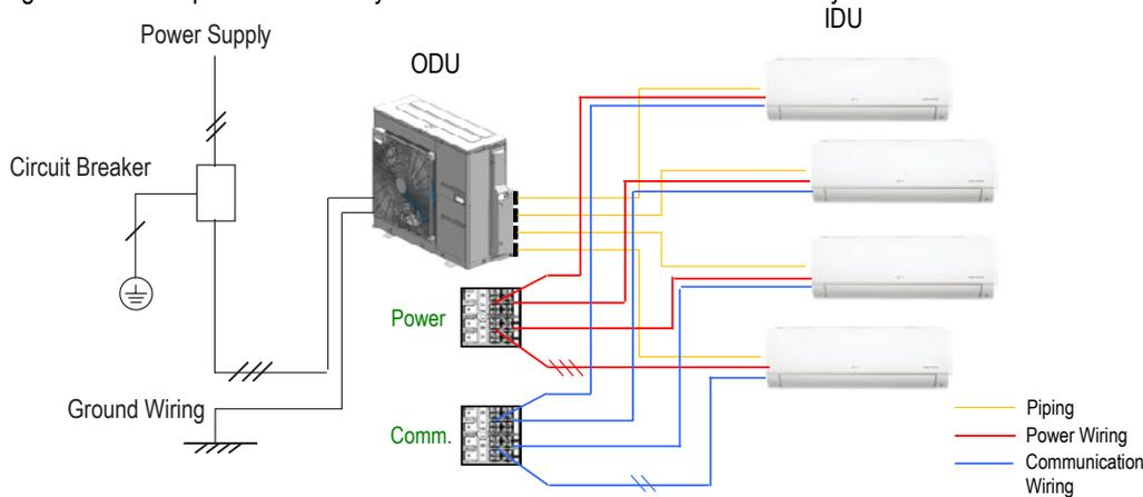
Figure 264: Example of a Multi F MAX System General Power / Communications System Schematic.
