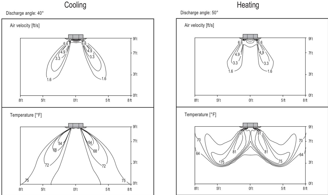
Figure 190: KNUDB091A Air Velocity and Temperature Distribution Charts.
