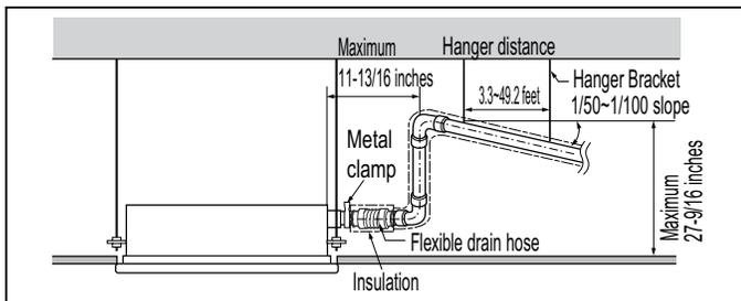
Figure 166: Indoor Unit Drain Piping.
