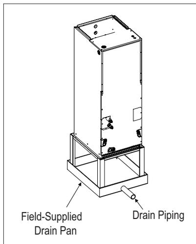
Figure 236: Typical Horizontal Left/Right Installation Drain System.
