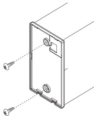
Figure 150: Installing / Removing the Controller.
