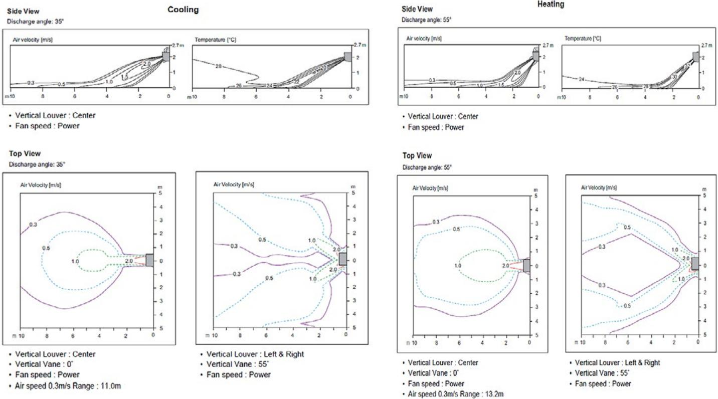
Figure 38: KNUAB181A Air Velocity and Temperature Distribution Charts.
