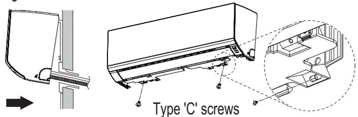
Figure 30: Removing the Filter Tabs.
