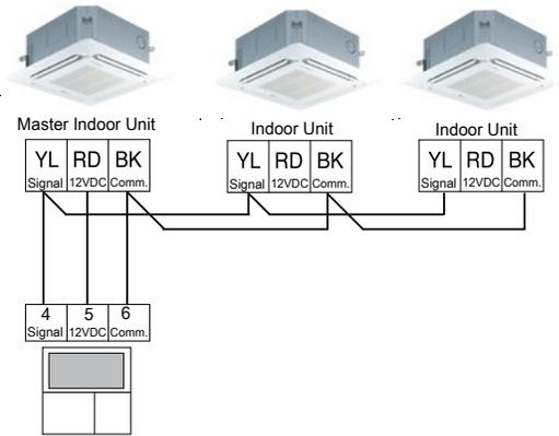
Figure 275: Example of Indoor Unit Group to Zone Controller Connections (CN-REMO).
