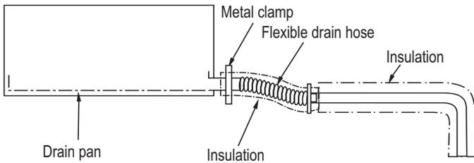
Figure 259: Diagram of an Indoor Unit with a Drain Pump.
