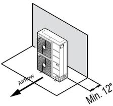
Single Unit—High Rear Wall with High Side Walls
