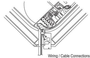
Figure 206: Simplified View of Indoor Unit to Outdoor Unit / Branch Distribution Unit Terminal Connections.
