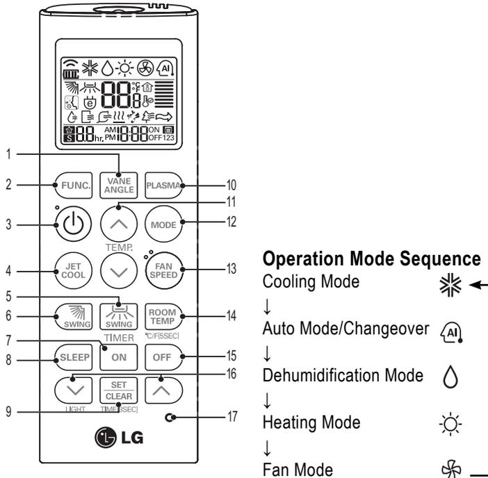
Table 94: AKB75735428 Wireless Handheld Controller Functions.<sup>1</sup>
