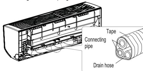
Figure 19: Piping Installed to the Right.
