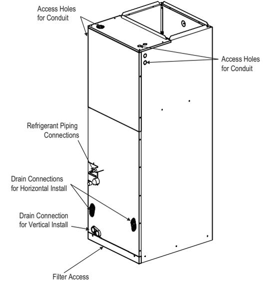
Figure 229: Location of Access Holes and Piping Connections.
