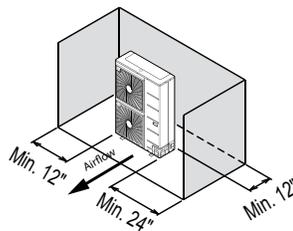
Single Unit—High Rear Wall with Building Overhang
