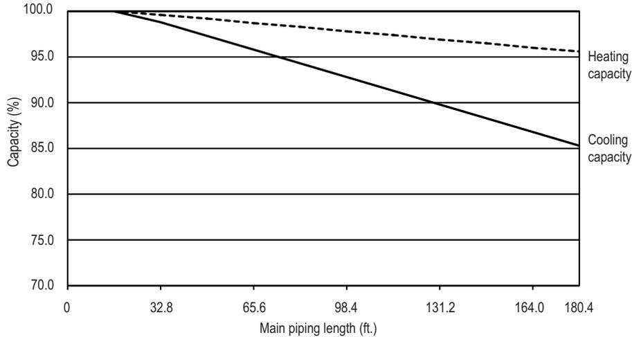
Table 118: Multi F MAX and Multi F MAX with LGRED Branch Distribution Unit to Indoor Unit Refrigerant Line Length Derates.
