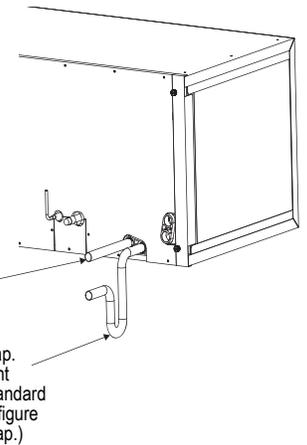
Figure 242: Insulating the Refrigerant Piping and Refrigerant Piping Connections.
