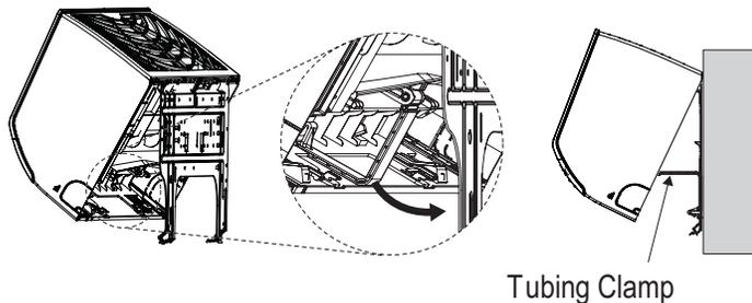
Figure 16: Removing the Frame Cover.
