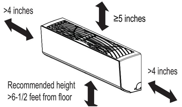
Figure 13: Preparing for Installation.
