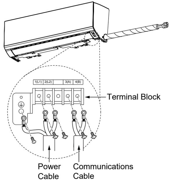
Figure 22: Simplified View of Art Cool Mirror Indoor Unit to Outdoor Unit / Branch Distribution Unit Terminal Connections.
