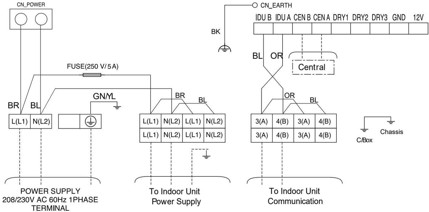
Connect the power wiring and communication wiring according to the number of indoor units installed.
