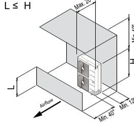
Side by Side—High Rear Wall and Low Front Wall with No Side Walls
