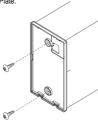
Figure 87: Installing / Removing the Controller.
