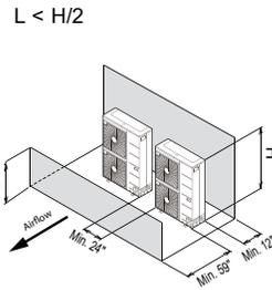
Side by Side—High Rear Wall and Low Front Wall with Building Overhang and No Side Walls
