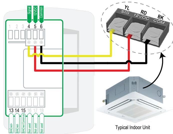
Figure 273: Another Example of Indoor Unit to Zone Controller Connection.
