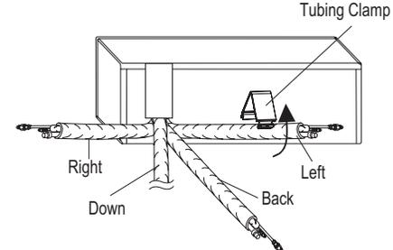
Figure 51: Piping Installed to the Left.
