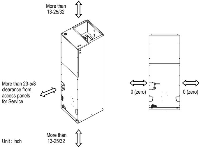
Figure 228: General and Duct Connection Dimensions.
