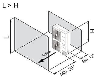
Single Unit—High Rear and Front Walls with Building Overhang
