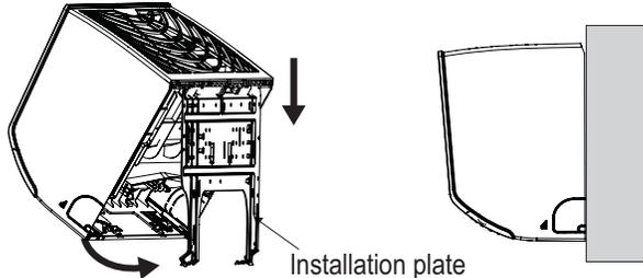
Figure 48: Accessing the Back of the Indoor Unit.
