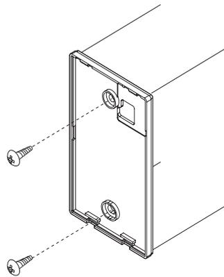
Figure 62: Installing / Removing the Controller.
