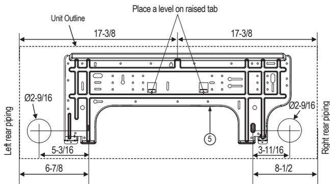
Figure 45: Installation Plate for KNUAB181A and KNMAB241A Units.
