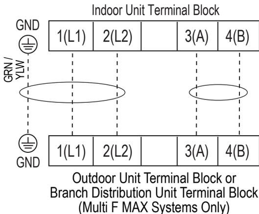
Figure 79: Connecting Power Wiring / Communications Cable.
