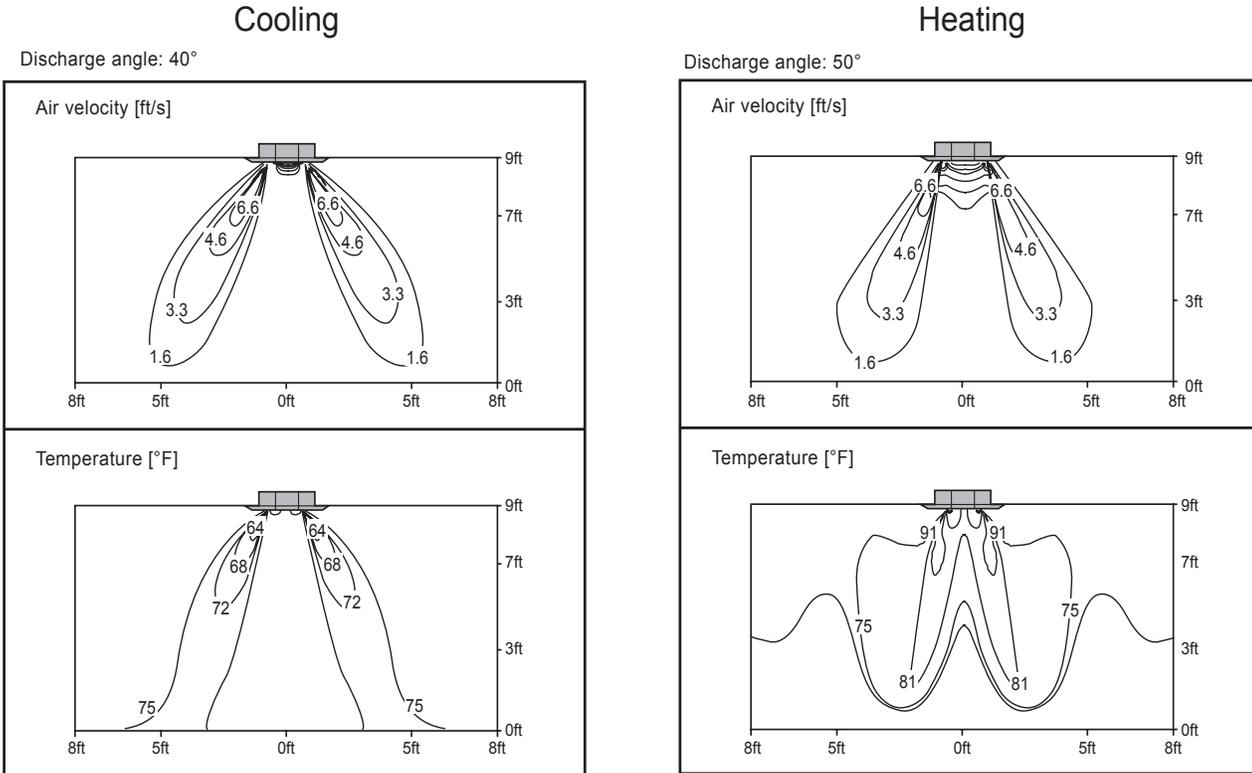
Figure 192: KNUDB181A Air Velocity and Temperature Distribution Charts.
