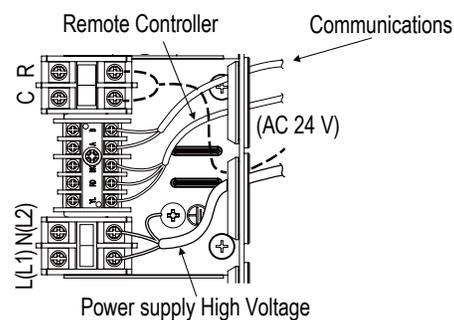
Figure 244: Indoor Unit to Outdoor Unit / Branch Distribution Unit (Multi F MAX systems only) Power Wiring / Communications Cable Connections.
