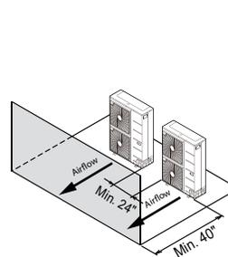
Side by Side—High Front Wall with Building Overhang and No Side or Rear Walls
