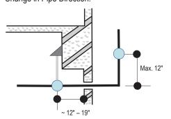
Figure 56: Pipe Support at Indoor Unit.
