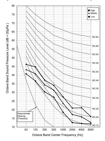
Figure 26: KNSLB301A Indoor Unit Sound Pressure Level Diagram.
