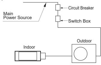
Figure 67: Power Wiring Example.
