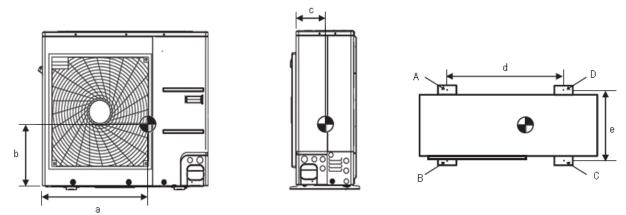
Figure 11: KUSXB361A, KUSXB421A, KUSXB481A, KUSXB601A Center of Gravity and Corner Weight Dimensions Diagram.
