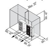
Figure 41: Proper Outdoor Unit Placement and Clearances When There Are Obstacles on the Discharge Side.
