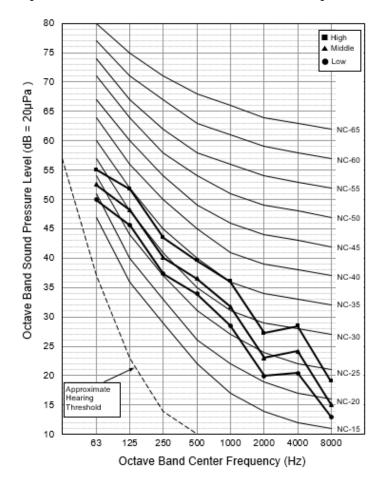
Figure 30: KNSLB601A Indoor Unit Sound Pressure Level Diagram.
