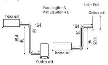
Figure 51: Typical KSSLB301A, KSSLB361A, KSSLB421A, KSSLB481A, KSSLB601A System Layout.
