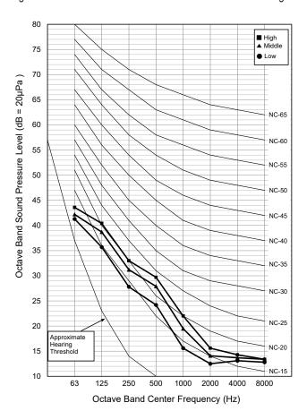
Figure 24: KNSLB181A Indoor Unit Sound Pressure Level Diagram.
