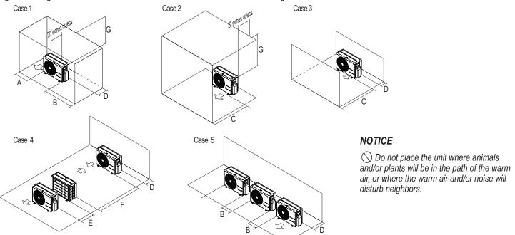
Table 60: Single Fan Outdoor Unit Service Access and Allowable Clearances Diagram Legend.
