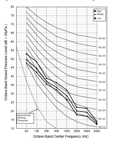
Figure 28: KNSLB421A Indoor Unit Sound Pressure Level Diagram.
