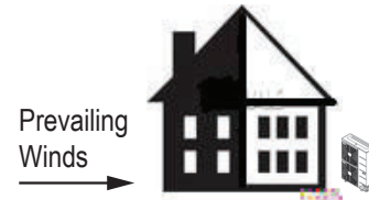
Figure 24: Leeward Side of the Building.
