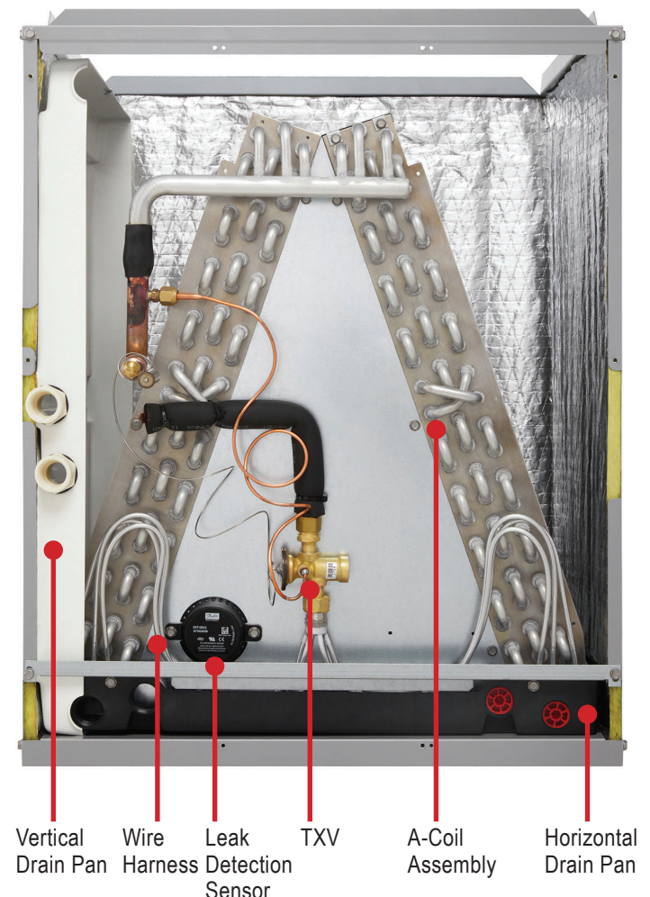
Figure 3: A-Coil Components.
