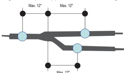
Figure 8: Pipe Support at Header Fitting.
