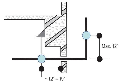
Figure 6: Pipe Support at Indoor Unit.
