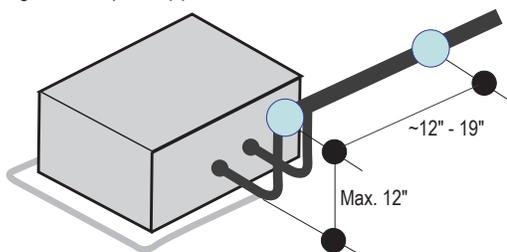
Figure 7: Pipe Support at Y-branch Fitting.
