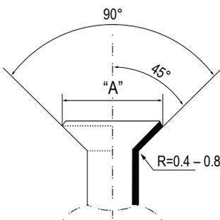
Flared Connection Dimensions / Tightening Torque.
