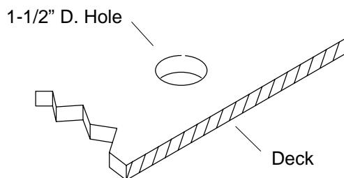
From above the deck, insert the threaded sleeve into the hole.
