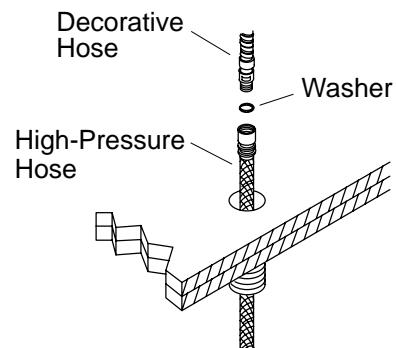
Thread the plastic shank into the threaded sleeve until tight. Do not overtighten.
