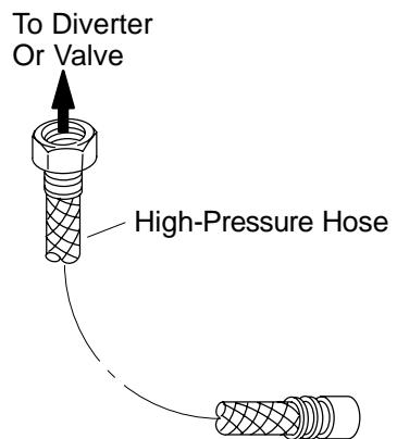
From the underside of the deck, insert the free end of the high pressure hose up through the threaded sleeve.
