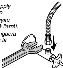
*Turn the water supply on, then check for leaks.*
