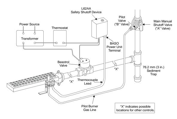
Figure 2: Typical L62AA Installation
