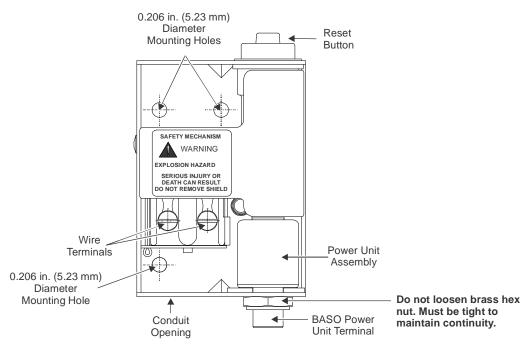
Figure 1: View of the L62AA Without the Cover
