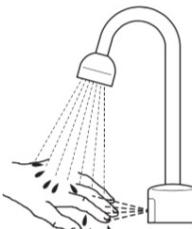
3. When hands are moved away from the OPTIMA® Sensor, the loss of reflected light initiates an electrical signal that deactivates the Solenoid Valve, shutting off the water flow. The Circuit then automatically resets and is ready for the next user.
