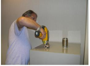
Pictured here the Plant Manager at Campbell Manufacturing, LLC. is performing a quality test on a lead free\* brass Slide Adapter using a Thermo Nitron XRF Analyzer. The Thermo Nitron XRF Analyzer is used to determine the lead content of a part to ensure lead free compliance. Employees conducting this test using this piece of equipment are professionally trained on the Thermo Nitron XRF Analyzer.
