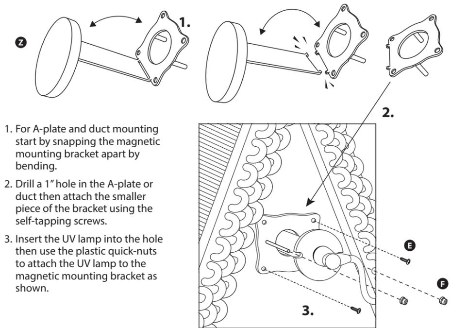
1. For A-plate and duct mounting start by snapping the magnetic mounting bracket apart by bending.
