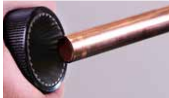
2. Deburr and remove all external sharp edges
