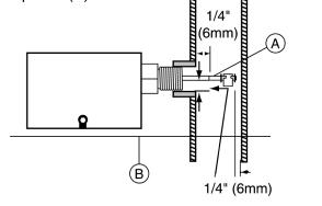
a. Apply pipe sealing compound on the probe threads (A).
