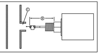
c. Using a 1-3/8" (35mm) open end wrench tighten the brass hex adapter (F) to 47 ft•lb (64 N•m).
