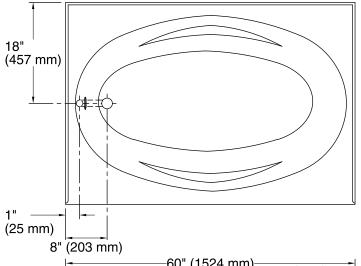
No change in measurements if connected with drain illustrated. (K-11677)
