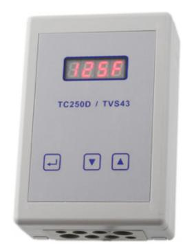
The TC250D is a proportional integral (PI) controller with an adjustable dead zone feature. The P action gives stability to the control loop but can result in some fluctuation around setpoint. The integral action (I) corrects the P error and brings the loop quickly back to setpoint.
