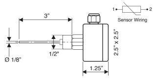
TS-ETS100 surface mounted pipe sensor. Thermistor NTC 1.8K
