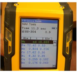
Pictured left: The Plant Manager of Campbell is performing a quality test on our stainless steel check valve using the Thermo Niton XRF Analyzer. The Niton XRF Analyzer is able to determine the lead content of the part to ensure it is lead free compliant; and also the grade of stainless the product is manufactured out of. In addition, the employees who conduct the tests using this piece of equipment are all professionally trained on how it works.
