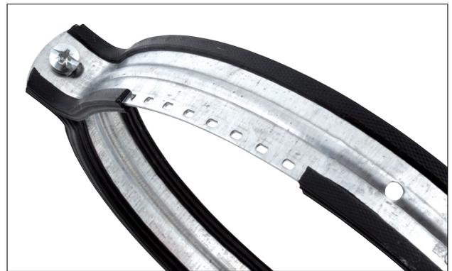
The rubber lining is formed around and through the steel band. It is conjoined with the steel and will not come off when sliding the spiral duct through the clamp.
