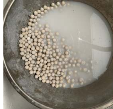
Figure 10: Neutralization media that has been rinsed with clean water
