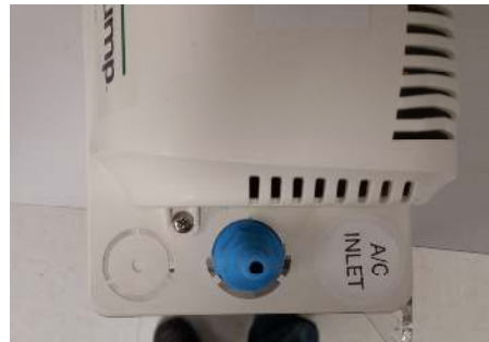
Figure 2: AC (Air Conditioning) inlet located beside check valve on top of NT1-P
