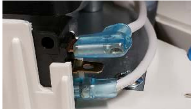
Fig. 4: High level float contacts in N.C. position
