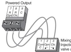
Mixing or Injection valve actuator
