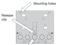
Conduit knockouts on back and bottom
