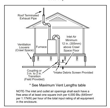
Figure 20. Equipment in Confined Space (Inlet Air from Ventilated Crawl Space and Outlet Air to Outside)
