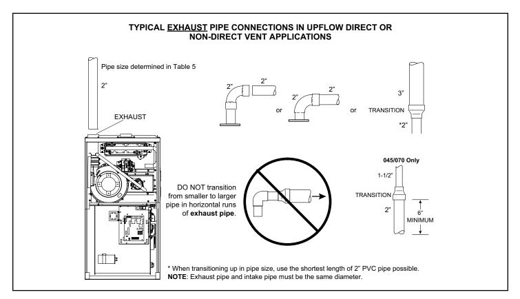
Figure 15. Typical Exhaust Pipe Connections in Upflow Direct or Non-Direct Vent Applications
