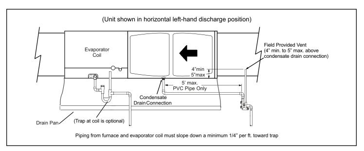
Figure 44. Furnace with Evaporator Coil Using a Separate Drain
