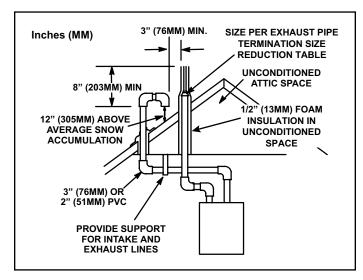
Figure 27. Direct Vent Roof Termination Kit (15F75 or 44J41)
