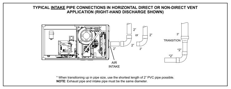
Figure 18. Typical Air Intake Pipe Connections in Horizontal Direct Vent Applications (Right Hand Discharge Shown)
