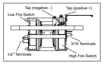
Figure 11. Combustion Air Pressure Switch
