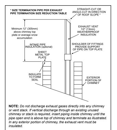
Figure 35. Non-Direct Vent Application Using Existing Chimney
