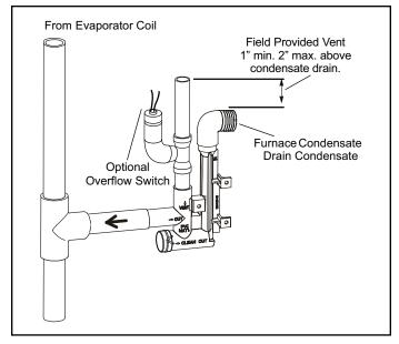
Figure 45. Condensate Trap With Optional Overflow Switch
