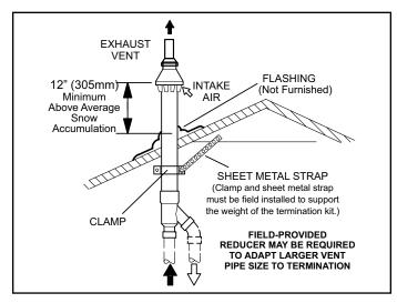
Figure 29. Direct Vent Concentric Rooftop Termination 71M80, 69M29 or 60L46 (US) 41W92 or 41W93 (Canada)
