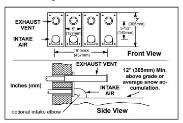
Figure 28. Optional Vent Termination for Multiple Unit Installation of Direct Vent Wall Termination
