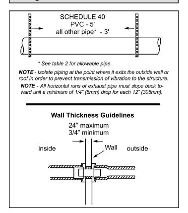
Figure 13. Piping Suspension Guidelines
