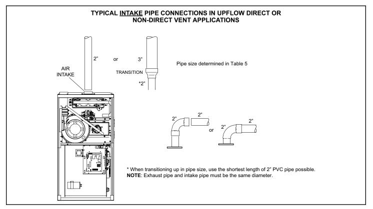
Figure 17. Typical Air Intake Pipe Connections in Upflow Direct Vent Applications
