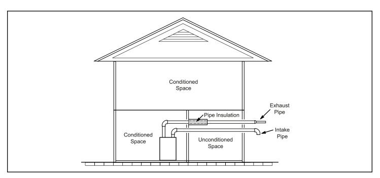
Figure 23. Insulating Exhaust Pipe in an Unconditioned Space
