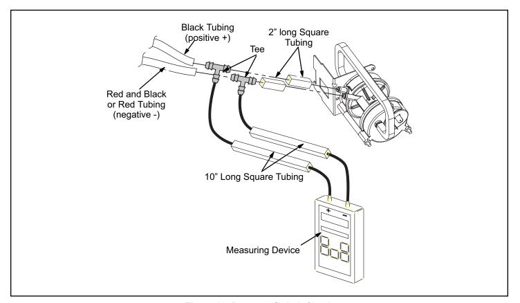
Figure 12. Pressure Switch Check
