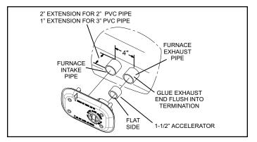
Figure 32. Flush-Mount Side Wall Termination 51W11
