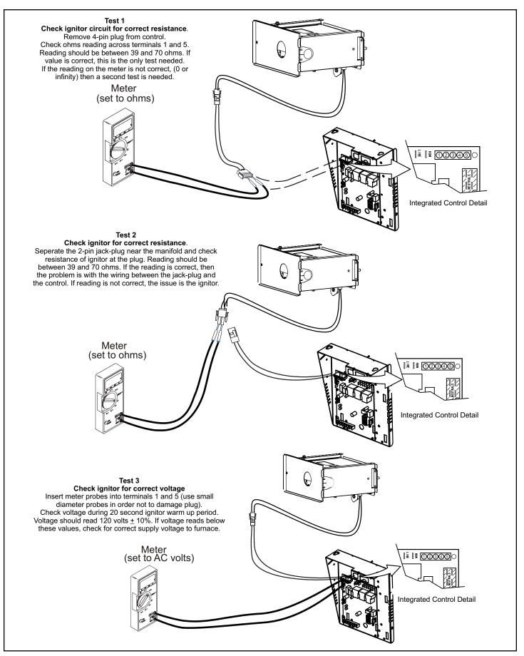
Figure 10. Ignitor Check
