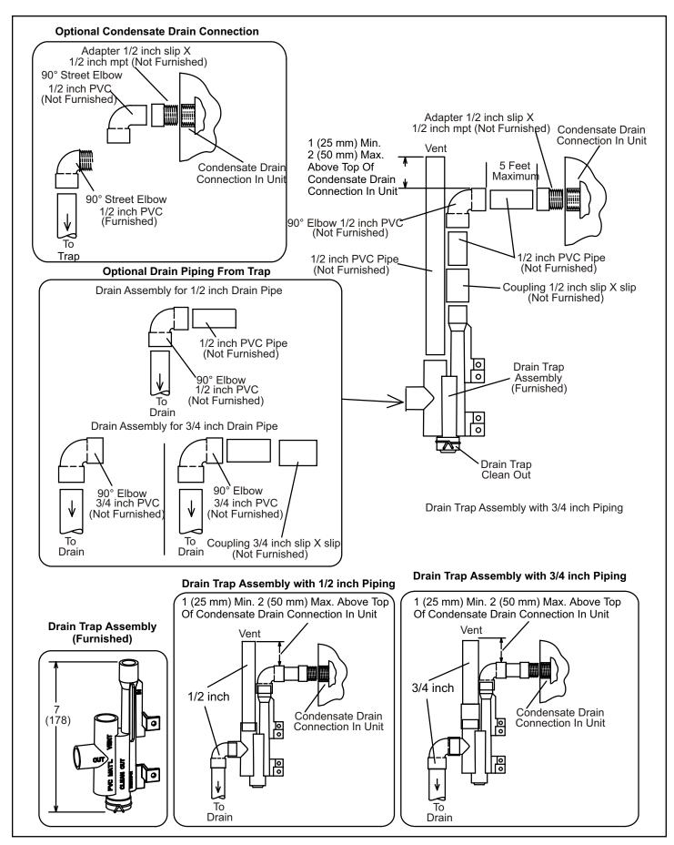
Figure 49. Trap / Drain Assembly Using 1/2" PVC or 3/4" PVC Cold End Header Box with 1/2 Drain Connection
