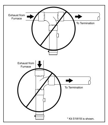
Figure 37. Crawl Space Vent Pipe Drain Trap
