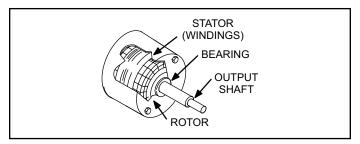
**Figure 6. Blower Motor Components**
