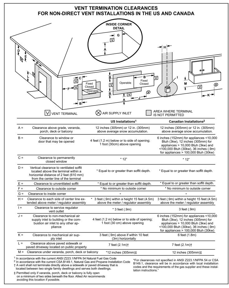
Figure 33. Vent Termination Clearances
