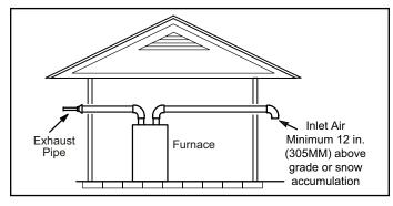
Figure 25. Exiting Exhaust and Intake Vent (no common pressure zone)
