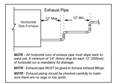
Figure 21. Horizontal Installation Offset Requirements
