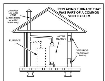
If the A97US2VX furnace replaces a furnace that was commonly vented with another gas appliance, the size of the existing vent pipe for that gas appliance must be checked. Without the heat of the original furnace flue products, the existing vent pipe is probably oversized for the single water heater or other appliance. The vent should be checked for proper draw with the remaining appliance.
