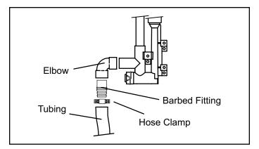
Figure 42. Field-Provided Drain Components
