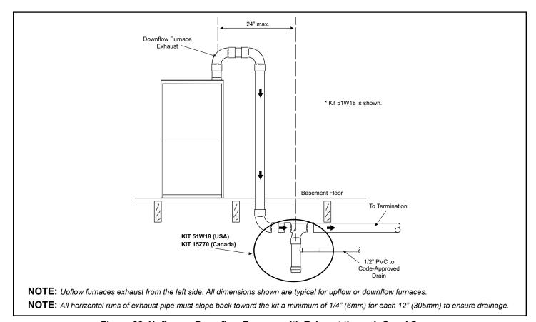
Figure 38. Upflow or Downflow Furnace with Exhaust through Crawl Space
