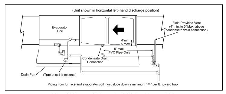
Figure 47. Furnace with Evaporator Coil Using a Common Drain
