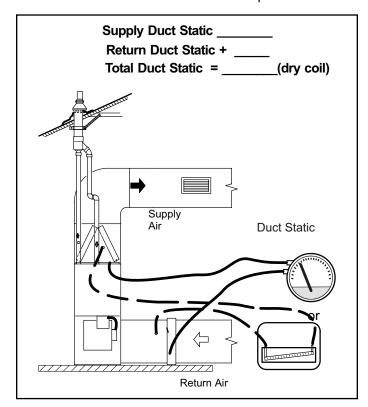
Figure 54. Static Pressure Test
