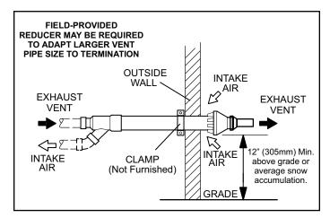
Figure 31. Direct Vent Concentric Wall Termination 71M80, 69M29 or 60L46 (US) 41W92 or 41W93 (Canada)
