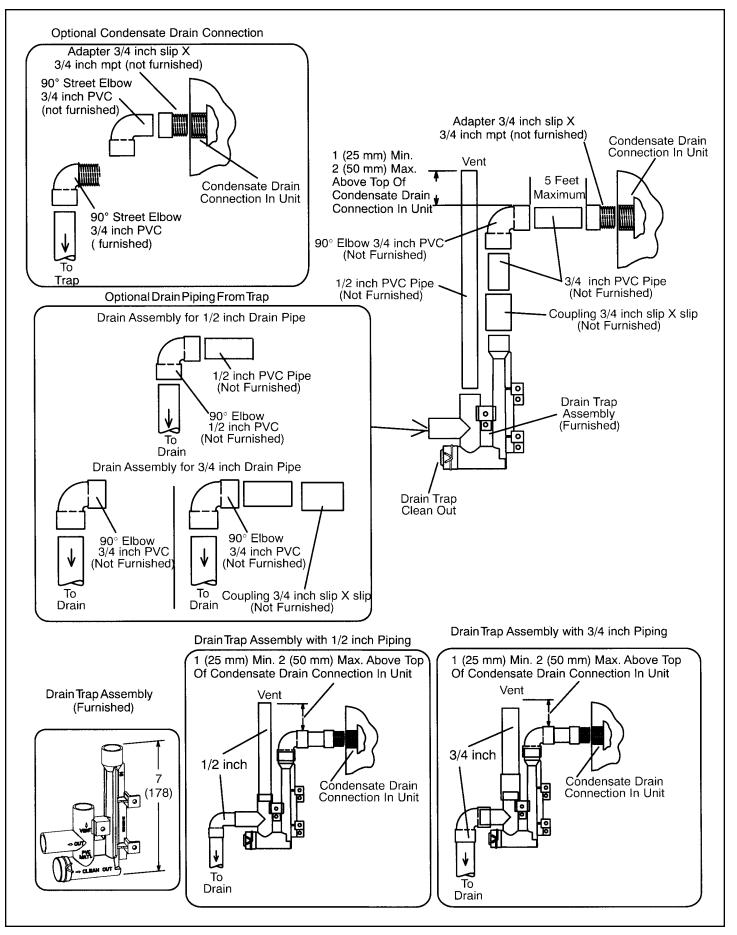
Figure 58. Trap / Drain Assembly Using 1/2" PVC or 3/4" PVC
