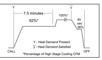
Figure 71. Indoor Blower Operation - Single Stage Cooling
