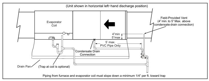
Figure 57. Furnace with Evaporator Coil Using a Common Drain
