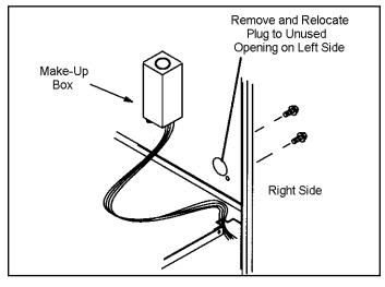
Figure 64. Interior Make-Up Box Installation
