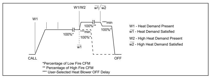
Figure 68. Indoor Blower Operation - 1st Stage-2nd Stage (W1/W2) Heat Call
