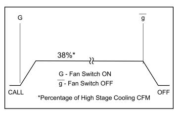
Figure 70. Indoor Blower Operation - Call for Fan
