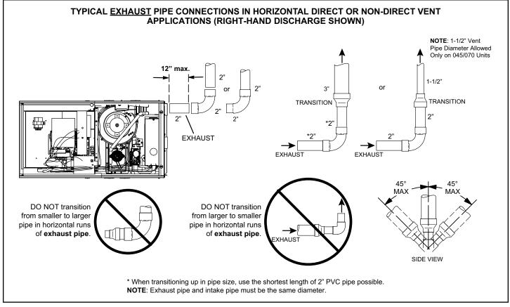
Figure 26. Typical Exhaust Pipe Connections in Horizontal Direct or Non-Direct Vent Applications (Right Hand Discharge Shown)
