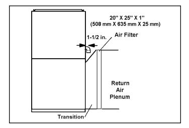
Figure 15. Side Return Air (with transition and filter)
