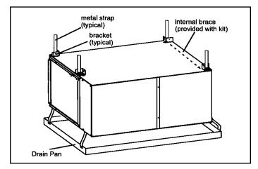
Figure 19. Typical Horizontal Application
