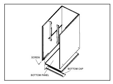
Figure 16. Removing the Bottom Panel
