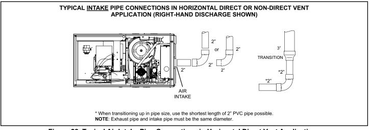
Figure 28. Typical Air Intake Pipe Connections in Horizontal Direct Vent Applications (Right Hand Discharge Shown)
