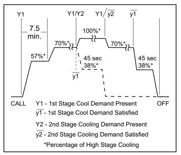
Figure 72. Indoor Blower Operation - Two Stage Cooling
