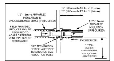
Figure 46. Non-Direct Vent Field Supplied Wall Termination
