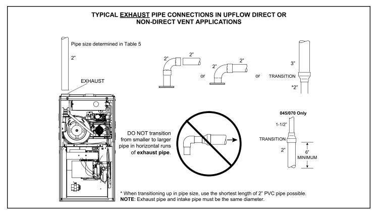
Figure 25. Typical Exhaust Pipe Connections in Upflow Direct or Non-Direct Vent Applications
