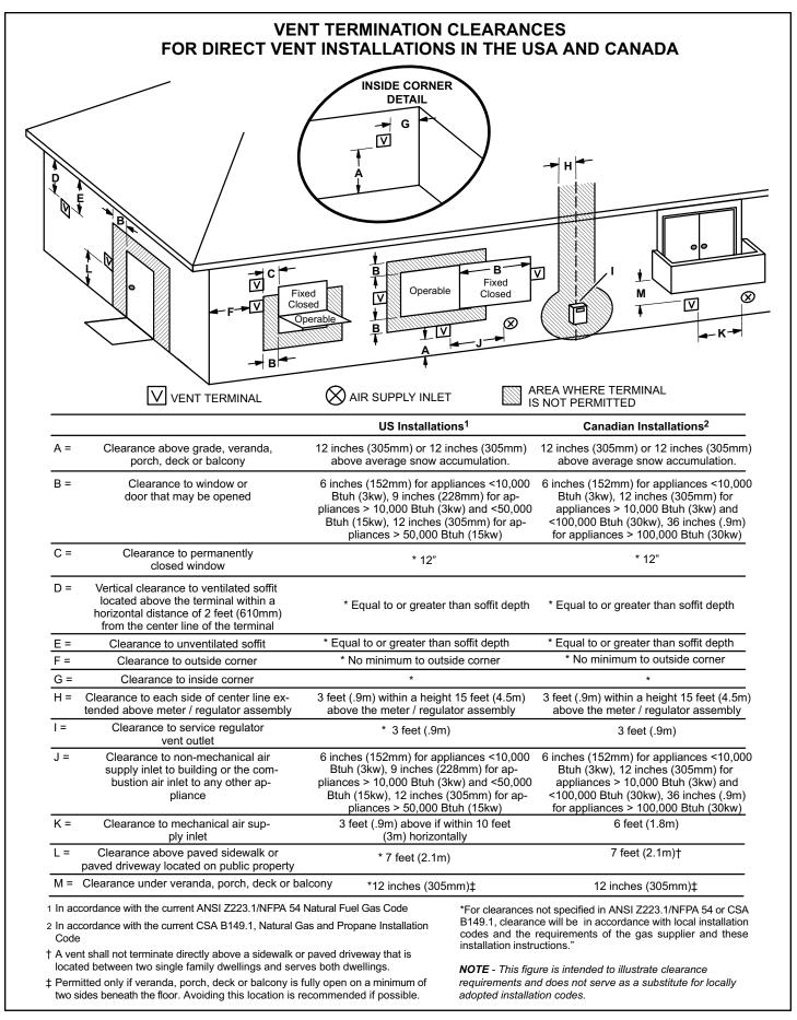
Figure 35. Vent Termination Clearances for Direct Vent Installations in the USA and Canada
