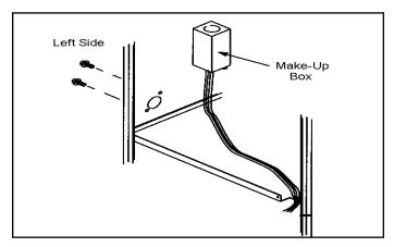
Figure 63. Interior Make-Up Box Installation
