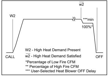
Figure 69. Indoor Blower Operation - High Heat (W2) Call
