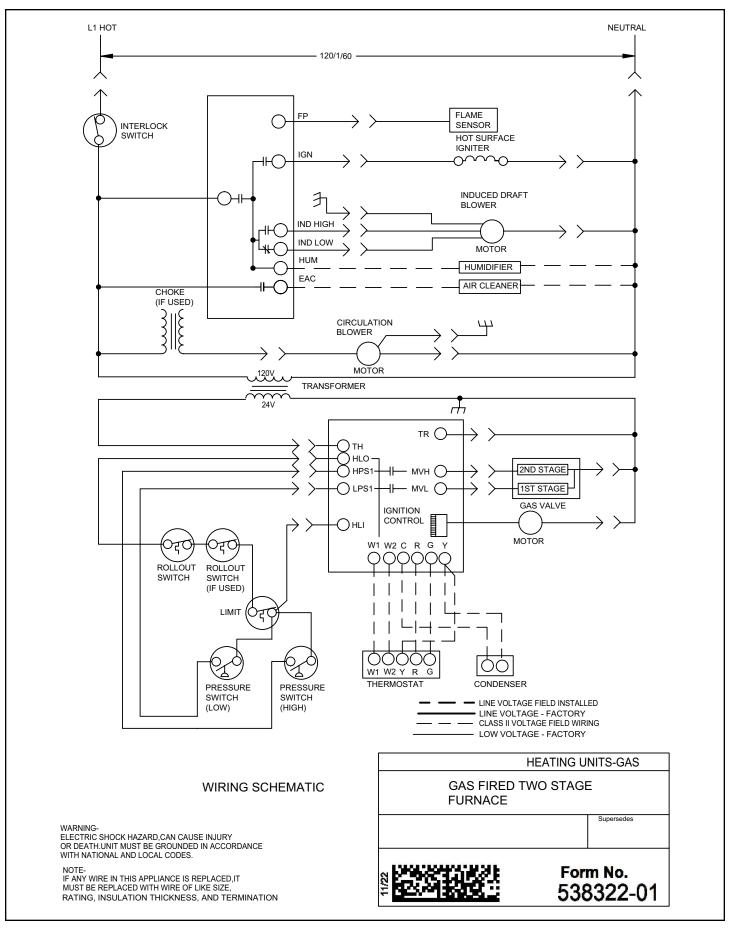
Figure 73. Typical Field Wiring Diagram
