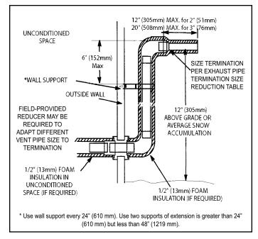
Figure 47. Non-Direct Vent Field Supplied Wall Termination Extended
