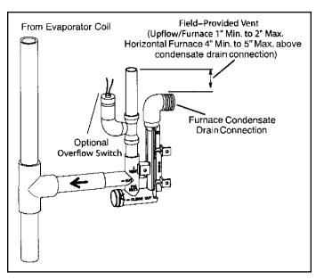
Figure 59. Condensate Trap with Optional Overflow Switch
