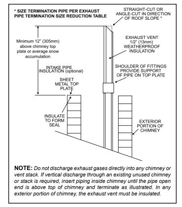
Figure 48. Non-Direct Vent Application Using Existing Chimney
