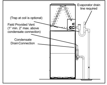
Figure 54. Furnace with Evaporator Coil Using a Separate Drain
