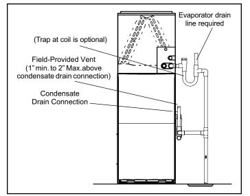
Figure 55. Furnace with Evaporator Coil Using a Separate Drain
