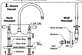
Ensure the mixer is orientated correctly, levers should rotate to point forward. After removing backnuts, place complete faucet through  $\emptyset1$ " holes at 7. 7/8" centers (do not remove unions from body) - product is fitted with straight unions, distance must be exact. Secure mixer with a suitable faucet wrench.
