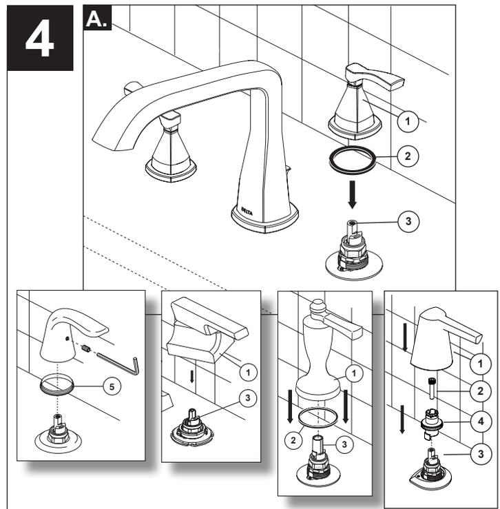
Install handles. **Make sure valve cartridge is in off position. On models with red/blue markings, be sure to use the correct handle assembly.**
