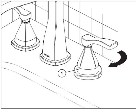
**B.** On some models, rotate handle base (1) clockwise, screwing it onto nut previously installed over the stem assembly until the handle base and gasket are firmly seated against deck and the handle base is aligned properly. **NOTE: If the handle needs to be adjusted, rotate handle base counter-clockwise until loose and pull-up to remove.**
