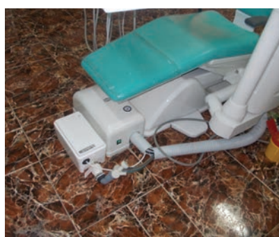
Dental chair equipped with Sanishower drain pumps
