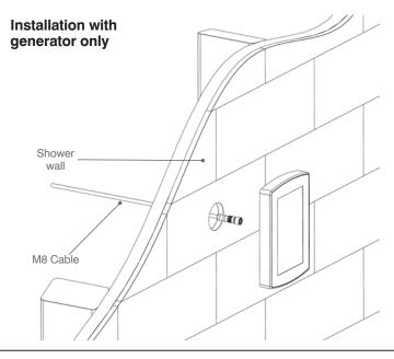
Route the M8 cable through the finished wall to the back side of the control. (The other end of the cable runs to the steam generator location.) NOTE: It is recommended to run the cable through electrical conduit. DO NOT STAPLE the cable!
