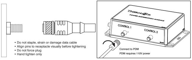
Connect the data cable to Power Distribution Module (PDM). (The other end of the cable runs to the back of the control in the shower location.)
