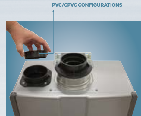
For PVC/CPVC configurations, the intake cap is removed and discarded. With this option, installers can use 3- or 4-inch PVC/CPVC pipe for the intake and exhaust.
