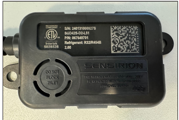
FIGURE 34. Example of Clear, Unobstructed Sensor Inlet
