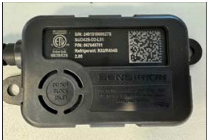
FIGURE 20. Example of Clear, Unobstructed Sensor Inlet
