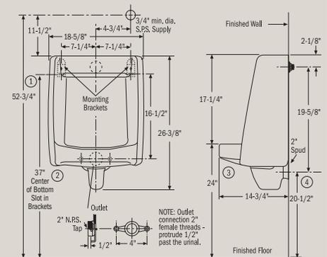
\*NOTE: Install this product according to the installation guide. Fixture dimensions are nominal and conform to tolerances in ASME Standard A112.19.2-2008/CSA B45.1-08.
