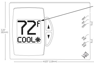
Easy to read LCD provides time, temperature and program information at a glance.
