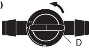
Turn refill adjuster dial (D) counter clockwise to fully closed.
