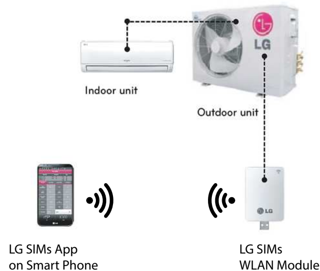
Figure 87: SIMS WLAN Module to DFS System Example.
