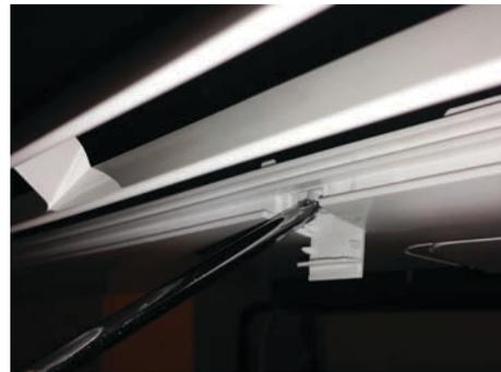
Figure 56: Removal (and Reattachment) of Bottom Panel
