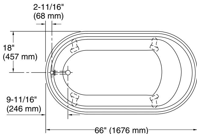
No change in measurements if connected with drain illustrated. (K-7178)
