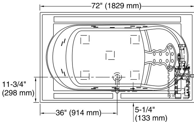
No change in measurement if connected with drain illustrated. (K-7161-AF)
