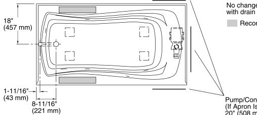
No change in measurements if connected with drain illustrated. (K-7161-AF)
