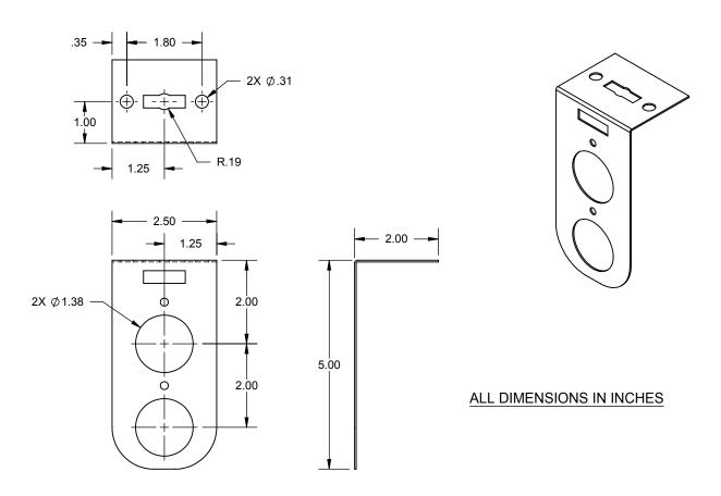
The HOLDRITE® #121-L is a 20 gage galvanized steel bracket that supports dual lines of 1/2", 3/4" or 1" Copper, PEX or CPVC tubing at 2" and 4" center line height. The hole pattern on the 90 $^{\circ}$  base allows for attachment to any flat surface. The bracket can also be suspended by 3/8" threaded rod.
