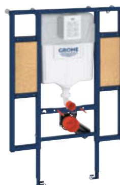
39 140 000 Rapid SL handicap for WC, flushing cistern GD 2 with small maintenance access 1.13 m installation height with fixing element for back support and bars, for WC bowls 70 cm projection
