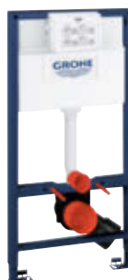
38 525 001 Rapid SL for WC with flushing cistern 3 – 6 l dual flush/start & stop/single flush, 1.00 m installation height connection from left/right/rear actuation from front/above
