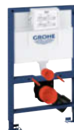
39 140 000 Rapid SL handicap for WC, flushing cistern GD 2 with small maintenance access 1.13 m installation height with fixing element for back support and bars, for WC bowls 70 cm projection
