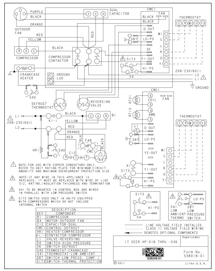
Figure 7. Wiring Diagram 018 - 036 Models
