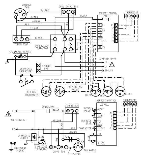
TPS = THERMAL PROTECTION SWITCH LO-PS = LOW PRESSURE SWITCH HI-PS = HIGH PRESSURE SWITCH
