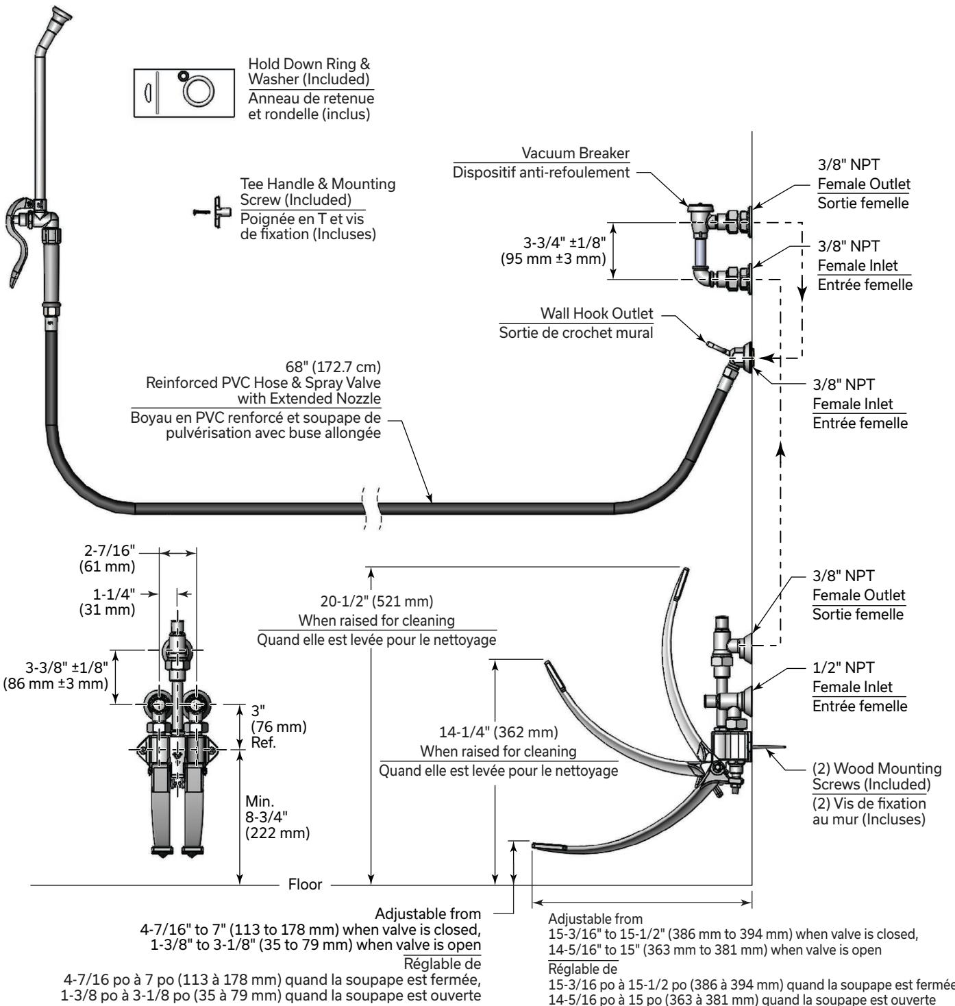
**NOTICE** All Pedal Position Dimensions are Based on Minimum Recommended Mounting Height of 8-3/4" (222 mm) Above Finished Floors.
