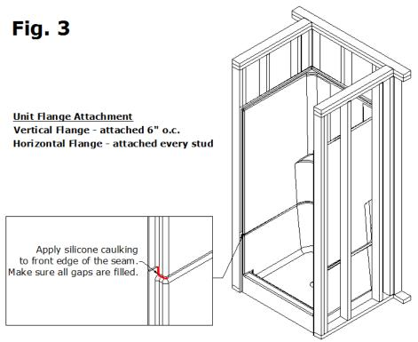
Apply silicone to the front seam and up the nailing flange where the wall section meets the base section. This will ensure that water cannot weep into the drywall from behind.
