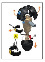
To purge the ferrous impurities in the steel DIRTMAG<sup>®</sup>, the flexible magnetic stack is removed from the brass dry-well and, with the system still running, the drain valve is opened. Aided by the system pressure, the dirt and ferrous impurities, including magnetite flushes out quickly and effectively.
