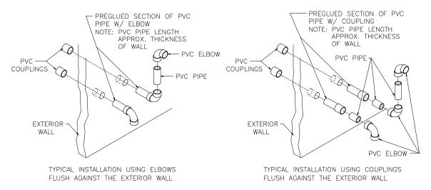
Figure 10: Typical Construction Details of Sidewall Vent and Air Intake
