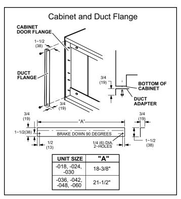
Figure 9. Cabinet and Duct Flange
