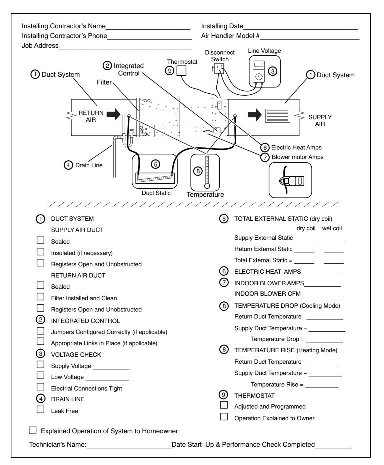
Figure 19. Start-up and Performance Checklist (Horizontal Configuration)
