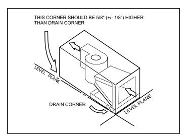
Figure 6. Sloping the Unit for Proper Drainage
