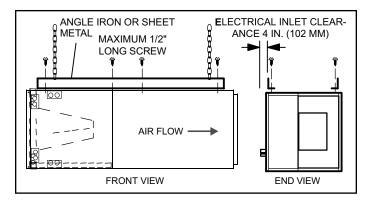
Figure 3. Suspending Horizontal Unit
