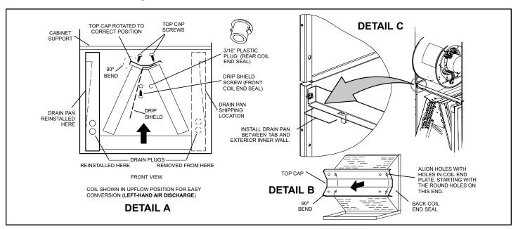
Figure 5. Field Modification for Left-Hand Discharge
