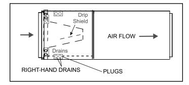
Figure 2. Right-Hand Discharge Configuration
