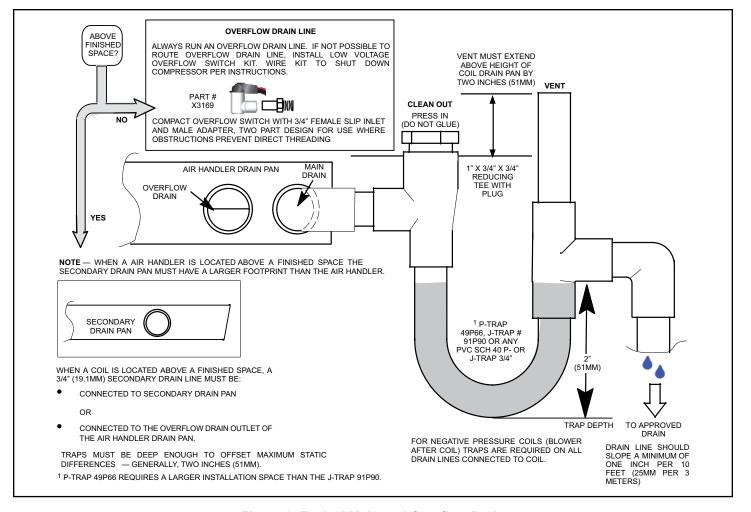
Figure 8. Typical Main and Overflow Drain
