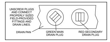
Figure 7. Drain Line Connections
