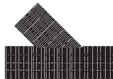
FABRICATED WYE (HORIZONTAL)
