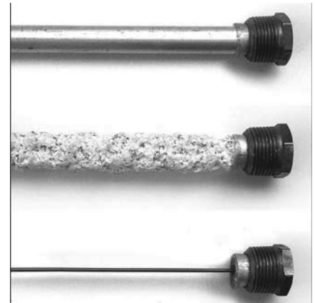
Figure 34 - Anode Rods from new (top) to partially depleted (middle) to fully depleted staged (bottom)
